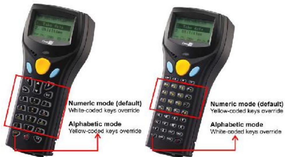
Figure 3: Keypad layout - 24-key (left), 39-key (right)
