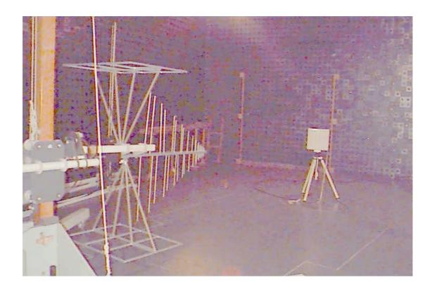
Photograph No.6 Radiated emissions measurement setup in the anechoic chamber, EUT view
