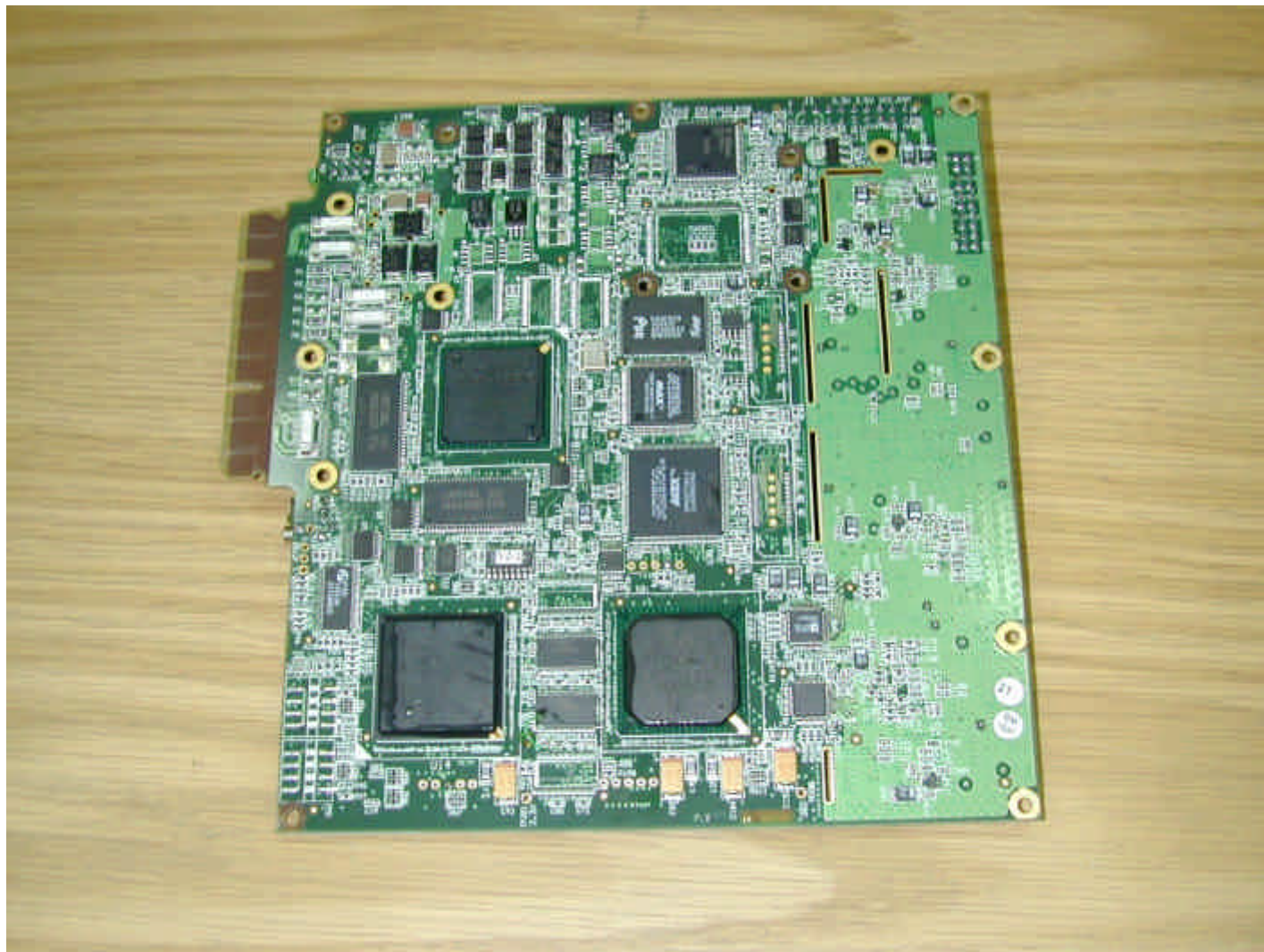
Photograph No.7 Winlink 582 outdoor radio terminal IF and digital PCB second side view
