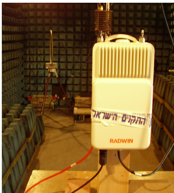
Photo #2. Radiated emissions test setup in anechoic chamber.
