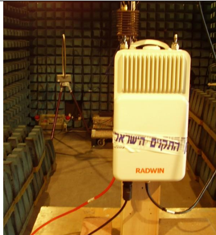
Photo #3. Radiated emissions test setup in anechoic chamber.
