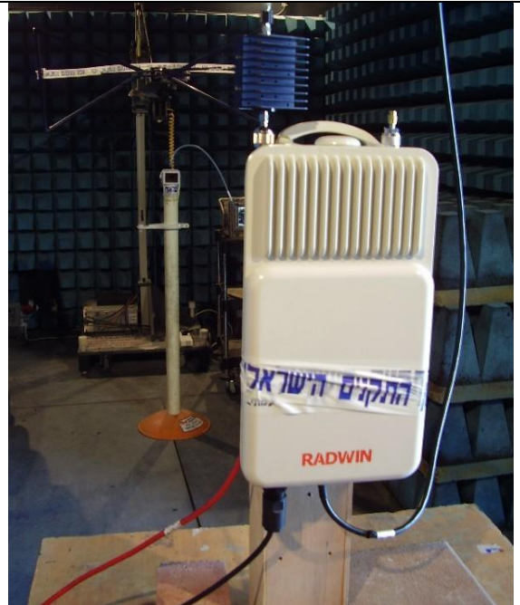
Photo #2. Radiated emissions test setup in anechoic chamber.
