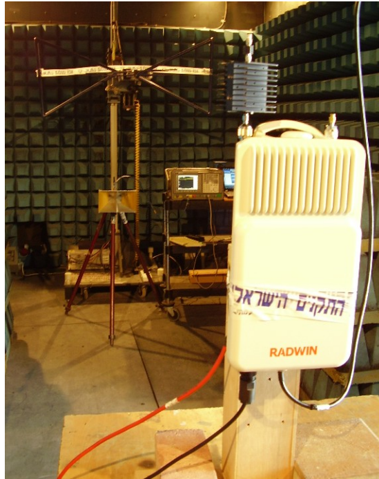
Photo #3. Radiated emissions test setup in anechoic chamber.
