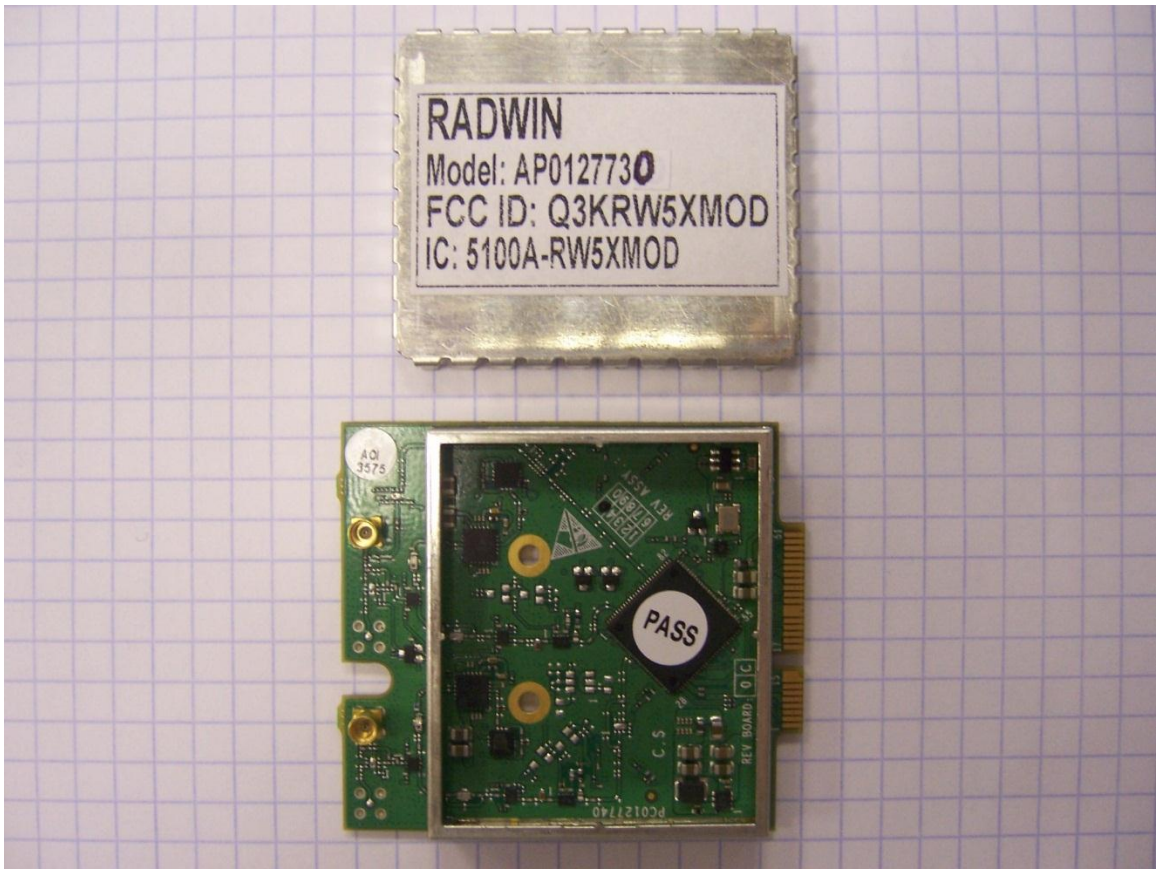
Photo 3: Front with shield removed
