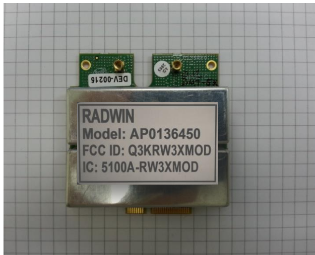
Module with the RF shielding and Label
