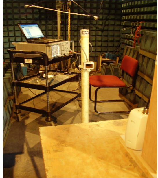
Photo #3. RE investigation setup in anechoic chamber.
