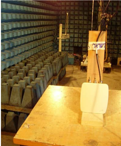
Photo #3. RE investigation setup in anechoic chamber.
