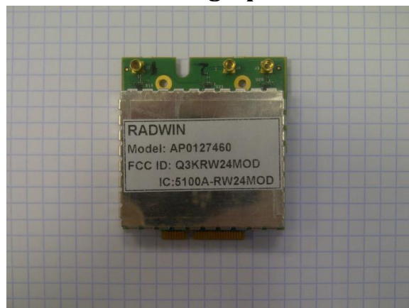
Module with the RF shielding and Label
