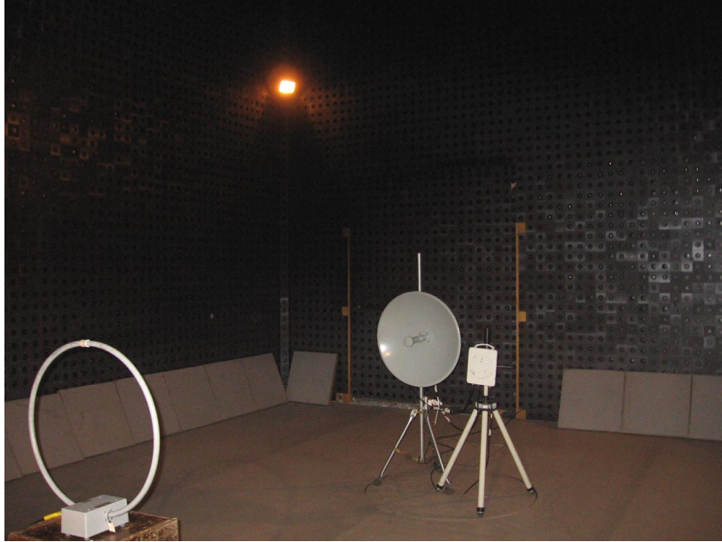
Photograph No.3 Radiated spurious emissions measurement setup below 30 MHz in the anechoic chamber, EUT with dish antenna
