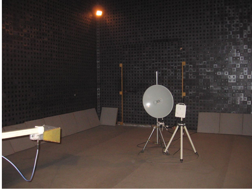
Photograph No.7 Radiated spurious emissions measurement setup in the anechoic chamber above 1000 MHz, EUT with dish antenna
