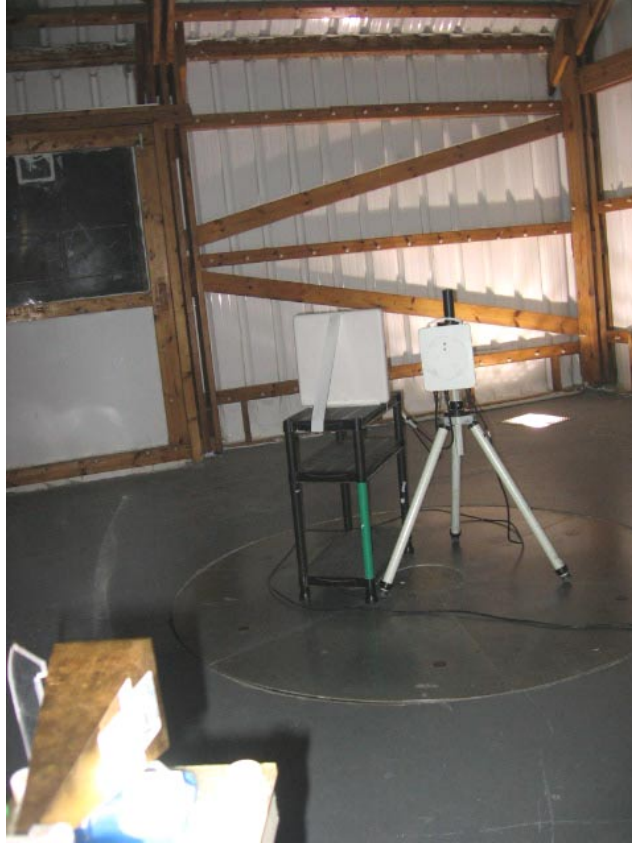
Photograph No.10 Radiated spurious emissions measurement setup at the OATS above 1000 MHz, EUT with flat antenna
