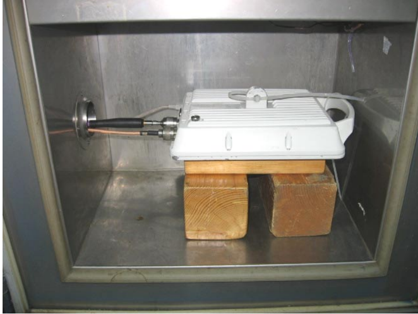
Photograph No.14 Frequency stability measurement setup
