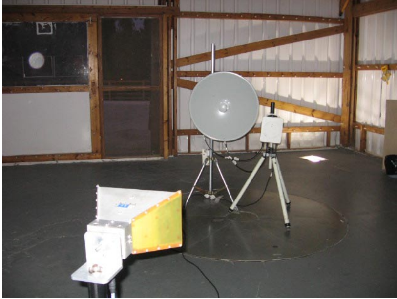
Photograph No.11 Radiated spurious emissions measurement setup at the OATS above 1000 MHz, EUT with dish antenna
