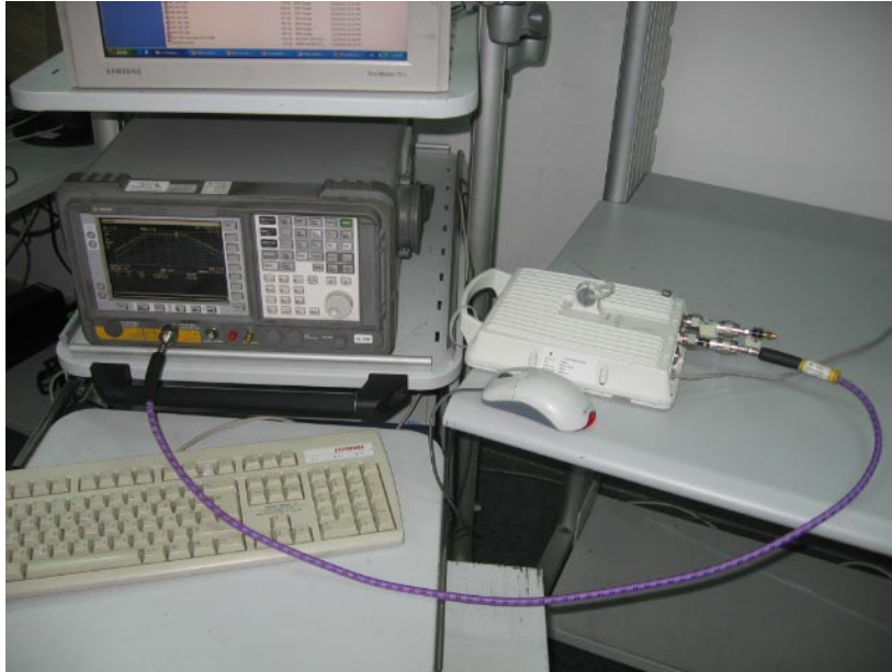
Photograph No.2 Peak excursion ratio and occupied bandwidth measurement setup
