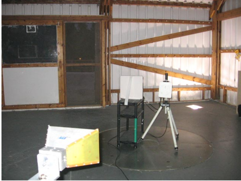
Photograph No.9 Radiated spurious emissions measurement setup at the OATS above 1000 MHz, EUT with flat antenna
