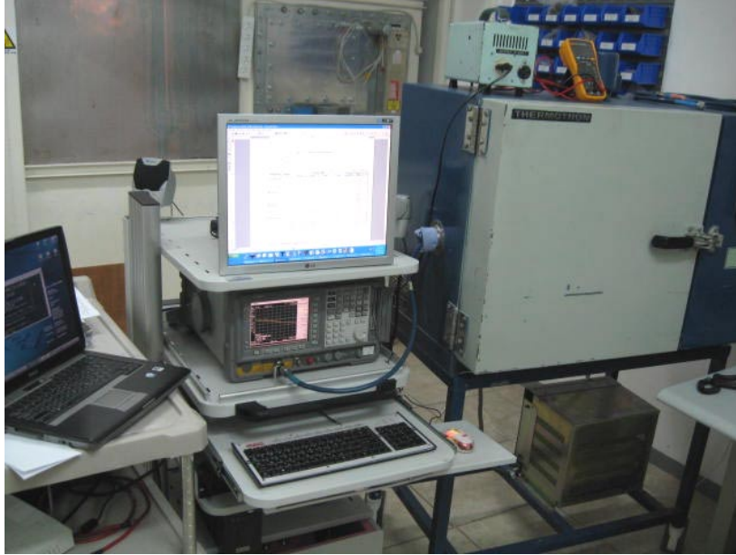
Photograph No.13 Frequency stability measurement setup
