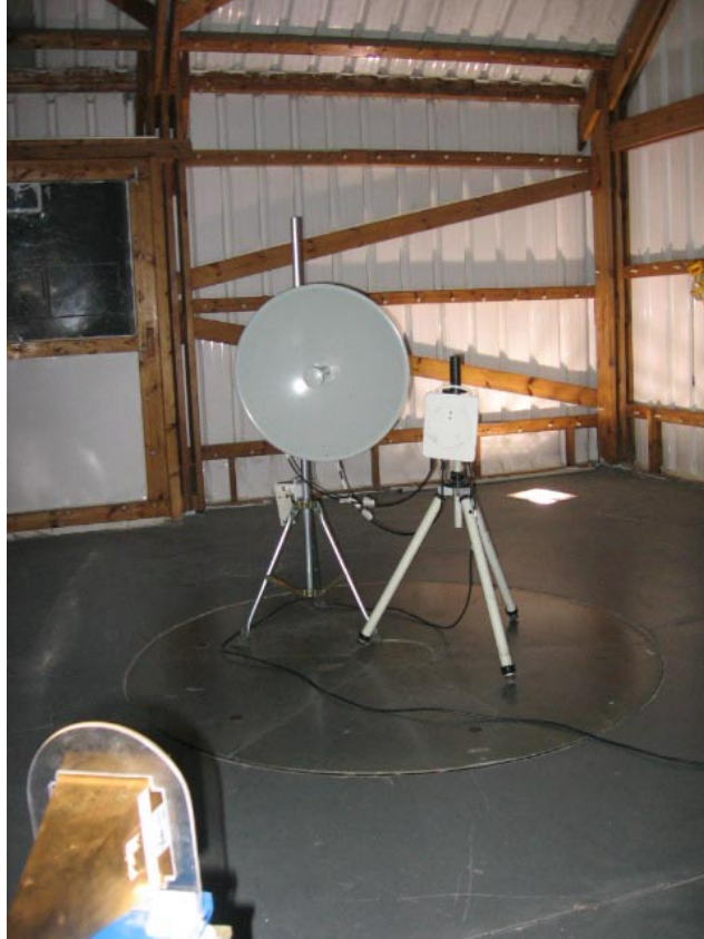
Photograph No.12 Radiated spurious emissions measurement setup at the OATS above 1000 MHz, EUT with dish antenna
