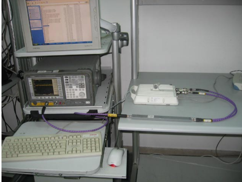
Photograph No.1 Peak output power measurement setup
