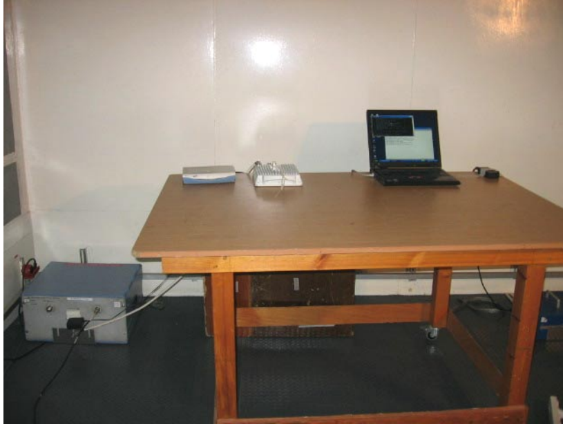
Photograph No.15 Conducted emission on power lines measurement setup
