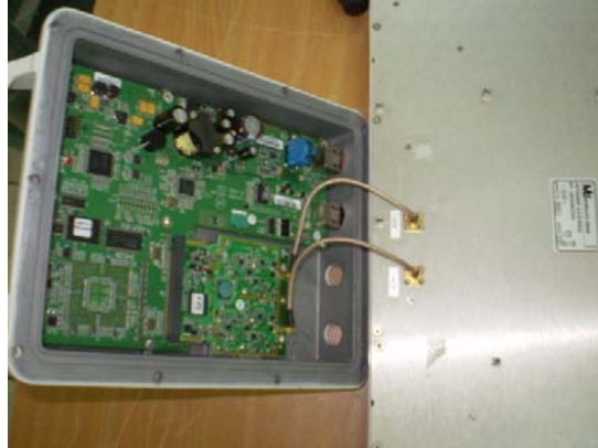
Photograph 7.7.2 Antenna assembly, integrated
