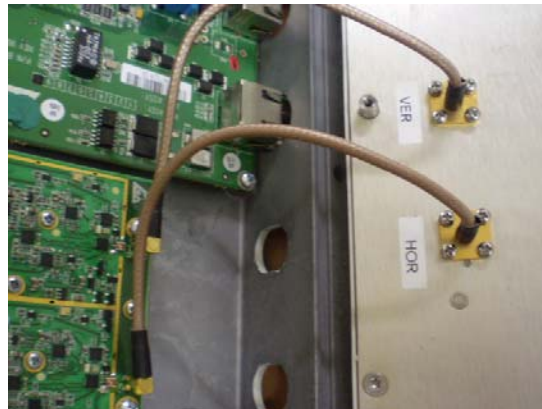
Photograph 7.7.3 Antenna assembly, integrated
