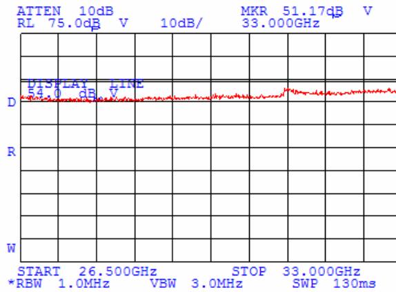
Plot 7.4.69 Radiated emission measurements from 26.5 to 33 GHz at the high carrier frequency
