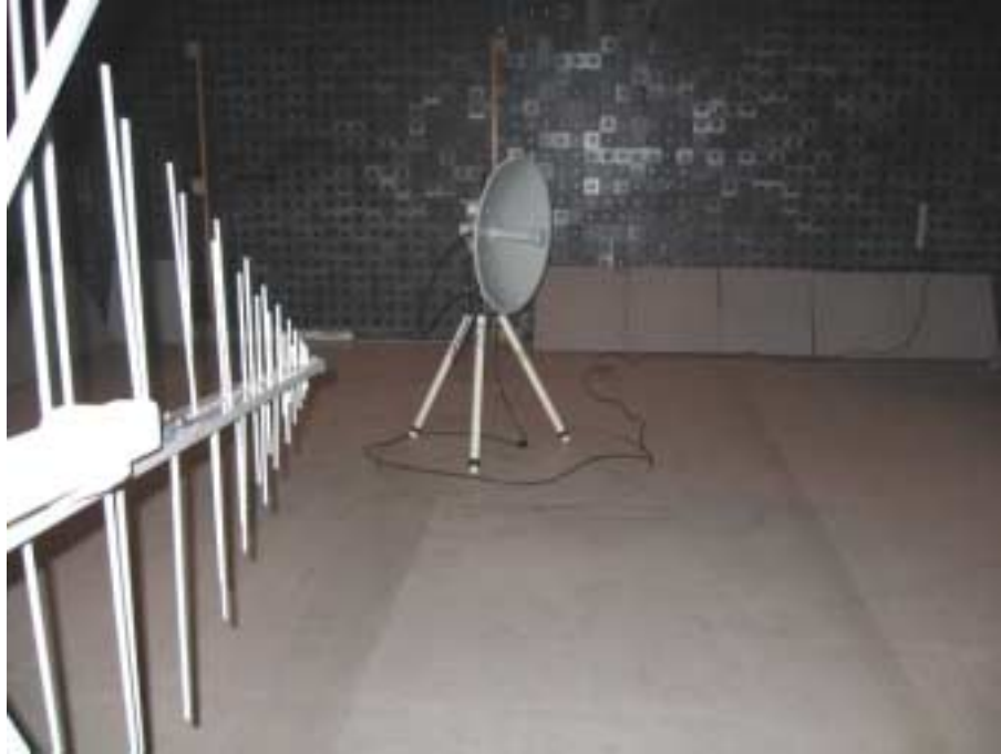
Photograph No.9 Radiated emissions measurement setup in the anechoic chamber with biconilog antenna, EUT with external dish antenna
