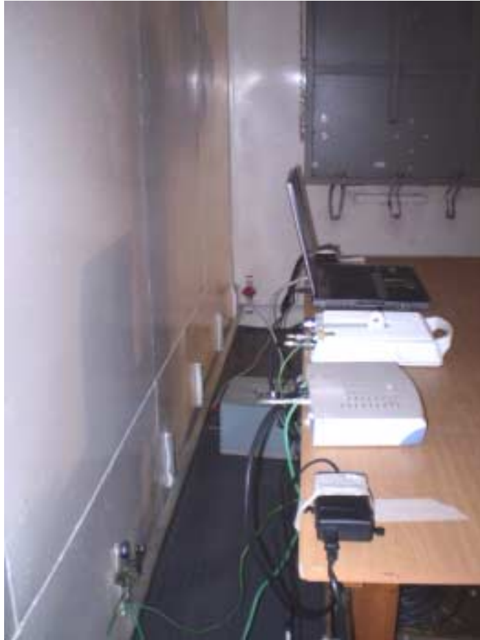
Photograph No.13 Conducted emission on power lines measurement setup
