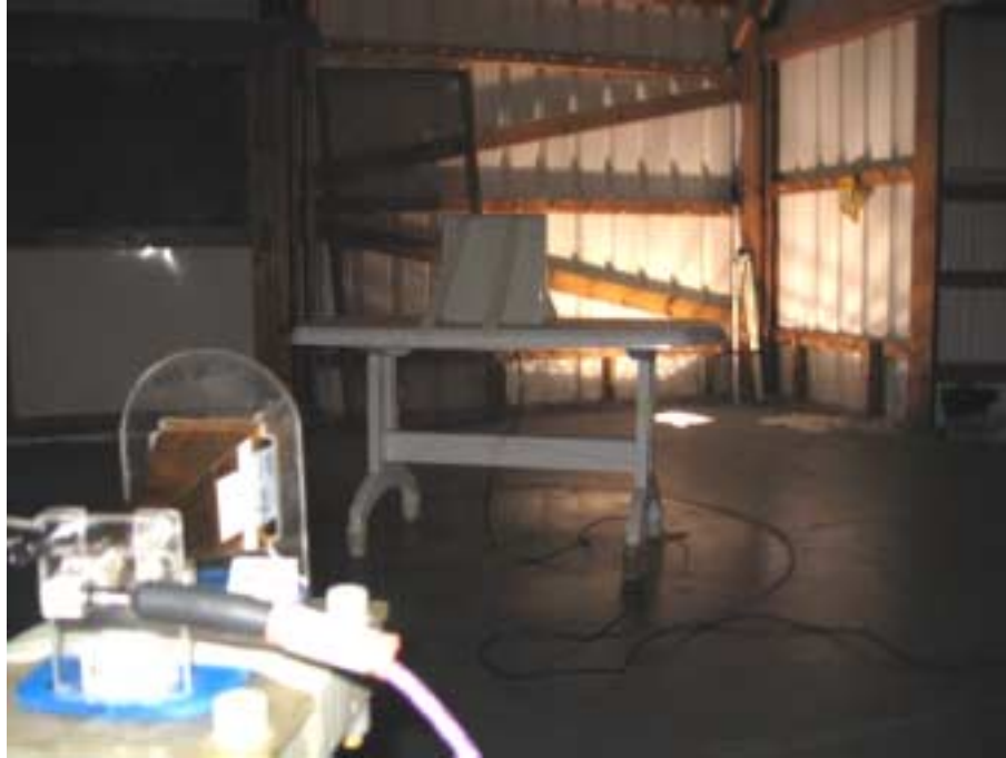
Photograph No.7 Radiated emissions measurement setup at the OATS with horn antenna, EUT with integrated flat antenna
