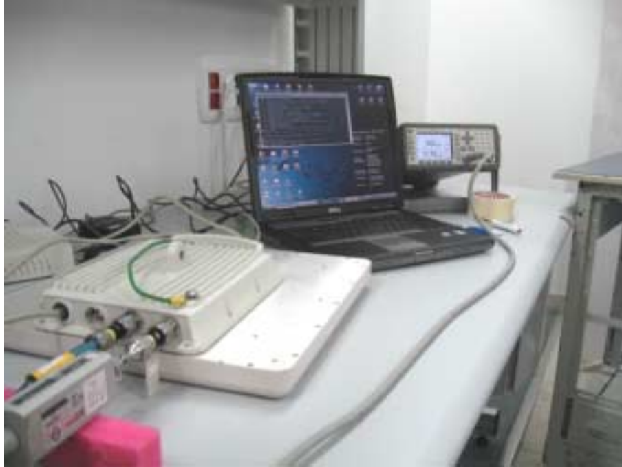
Photograph No.1 Peak output power measurement setup
