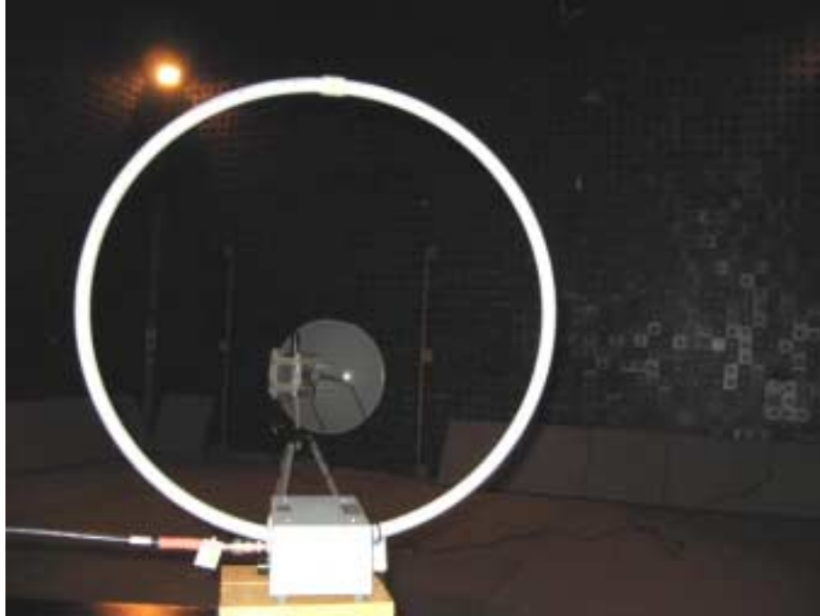
Photograph No.8 Radiated emissions measurement setup in the anechoic chamber with loop antenna, EUT with external dish antenna
