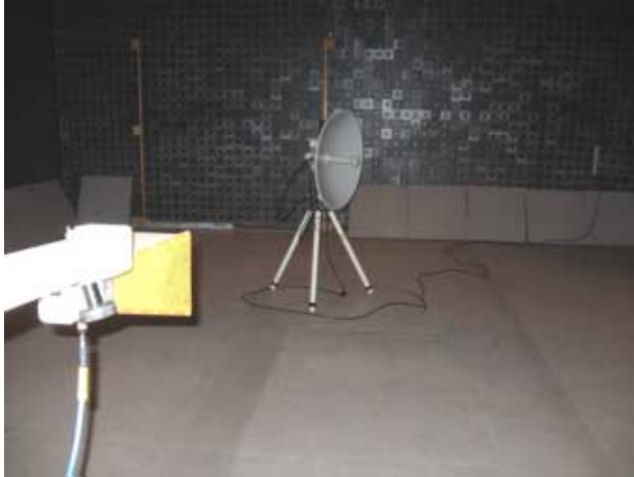
Photograph No.10 Radiated emissions measurement setup in the anechoic chamber with double ridged guide antenna, EUT with external dish antenna
