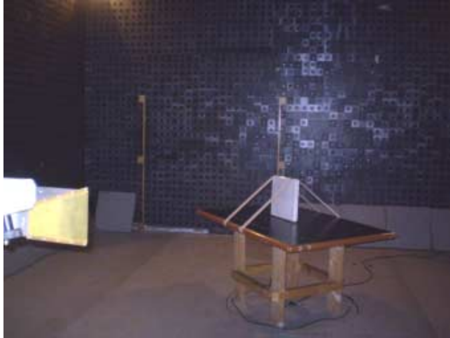
Photograph No.5 Radiated emissions measurement setup in the anechoic chamber with double ridged guide antenna, EUT with integrated flat antenna
