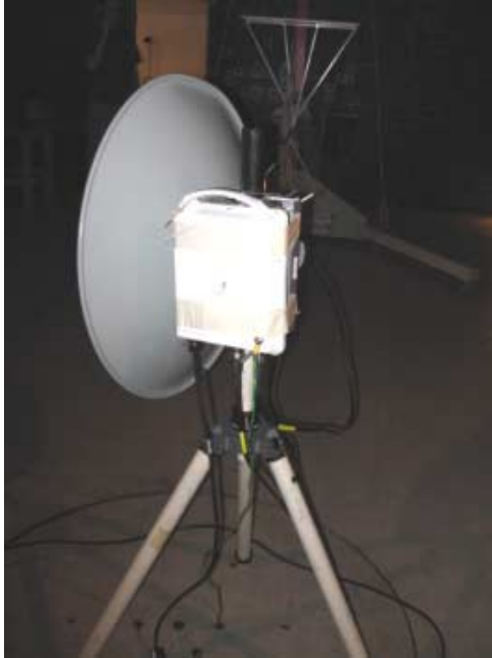
Photograph No.11 Radiated emissions measurement setup in the anechoic chamber, EUT with external dish antenna close view
