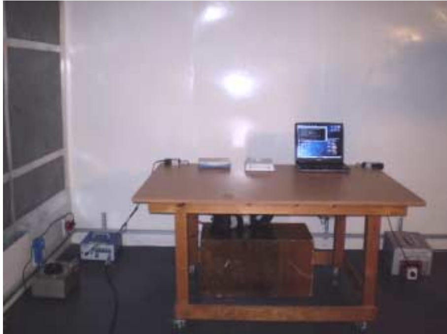
Photograph No.12 Conducted emission on power lines measurement setup
