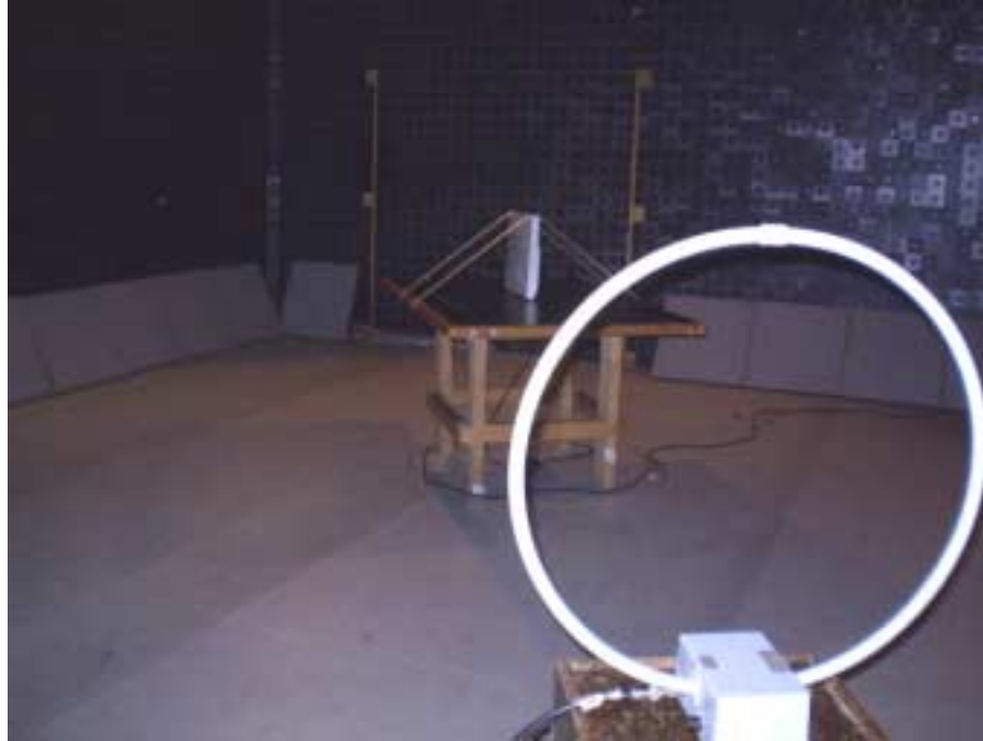
Photograph No.3 Radiated emissions measurement setup in the anechoic chamber with loop antenna, EUT with integrated flat antenna
