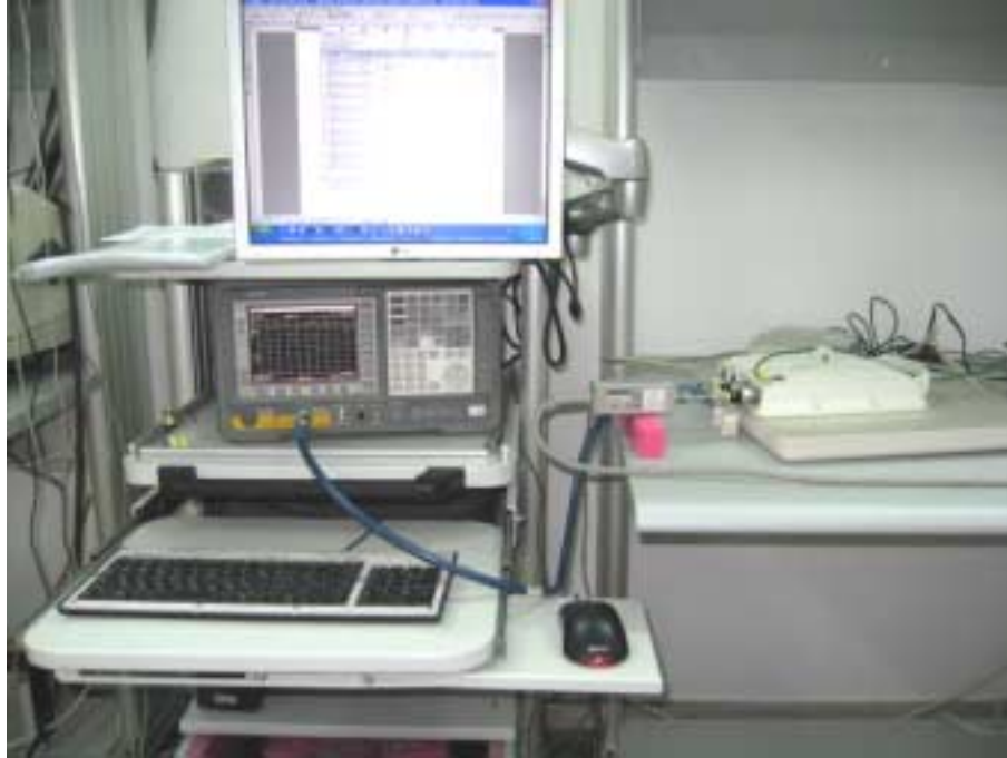
Photograph No.2 Occupied bandwidth, peak spectral power density, spurious emissions measurement setup
