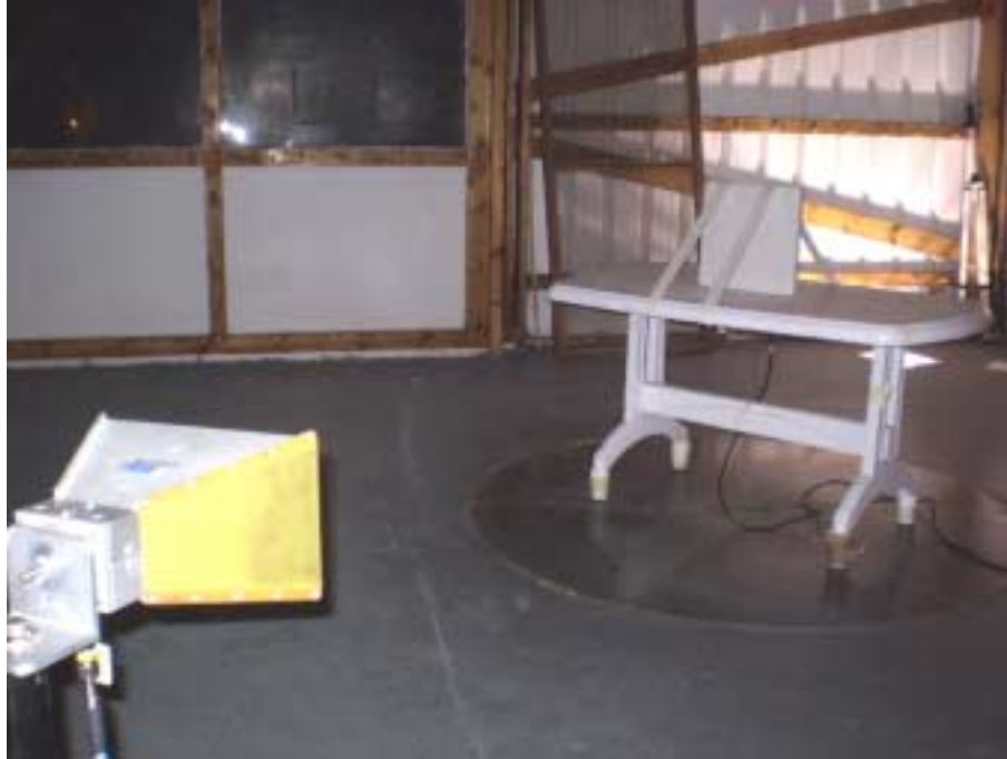
Photograph No.6 Radiated emissions measurement setup at the OATS with double ridged guide antenna, EUT with integrated flat antenna
