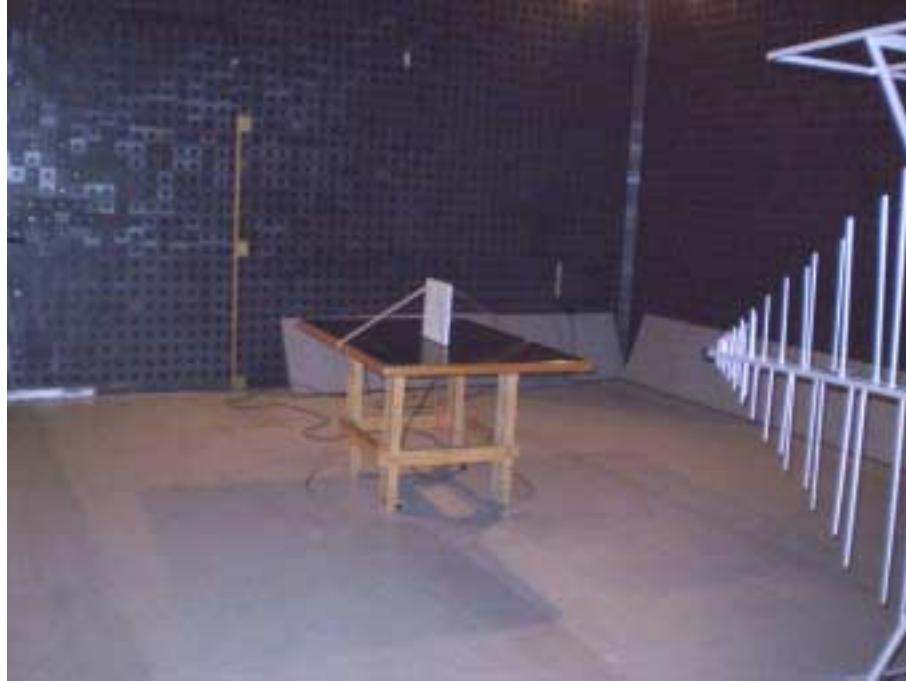
Photograph No.4 Radiated emissions measurement setup in the anechoic chamber with biconilog antenna, EUT with integrated flat antenna
