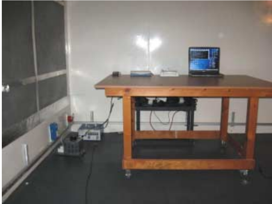
Photograph No.11 Conducted emission on power lines measurement setup
