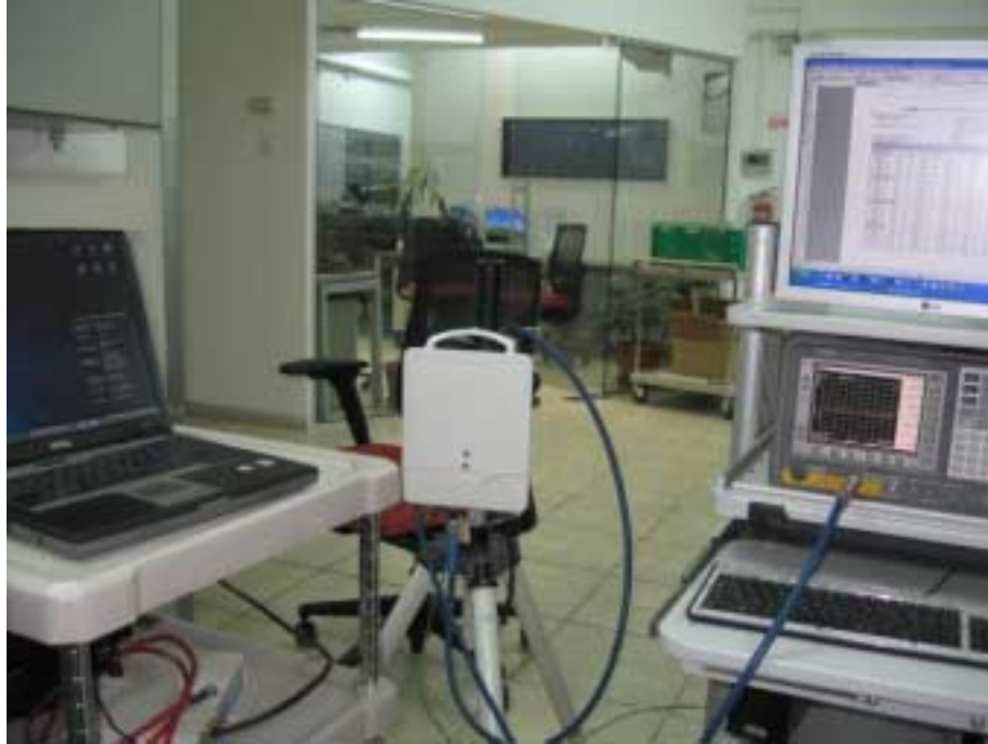
Photograph No.1 Peak output power, peak excursion ratio, spurious emissions measurement setup
