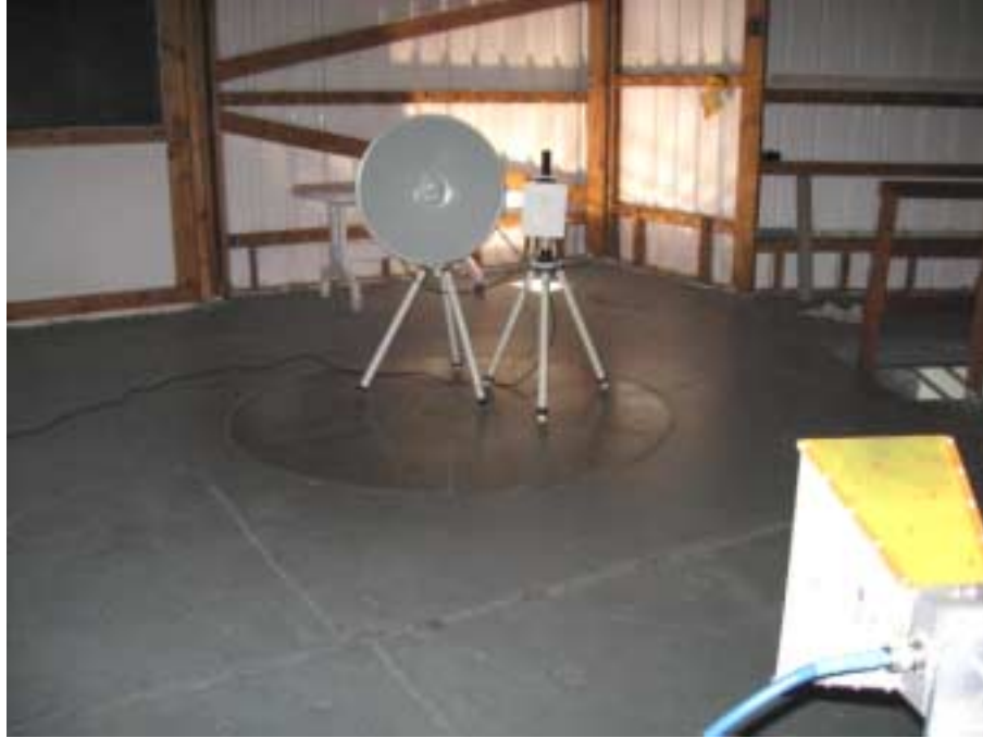
Photograph No.9 Radiated emissions measurement setup at the OATS with double ridged guide antenna, EUT with dish antenna
