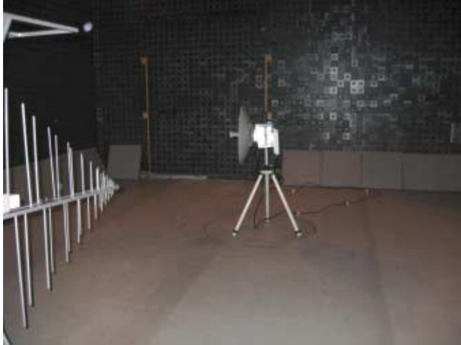
Photograph No.7 Radiated emissions measurement setup in the anechoic chamber with biconilog antenna, EUT with dish antenna
