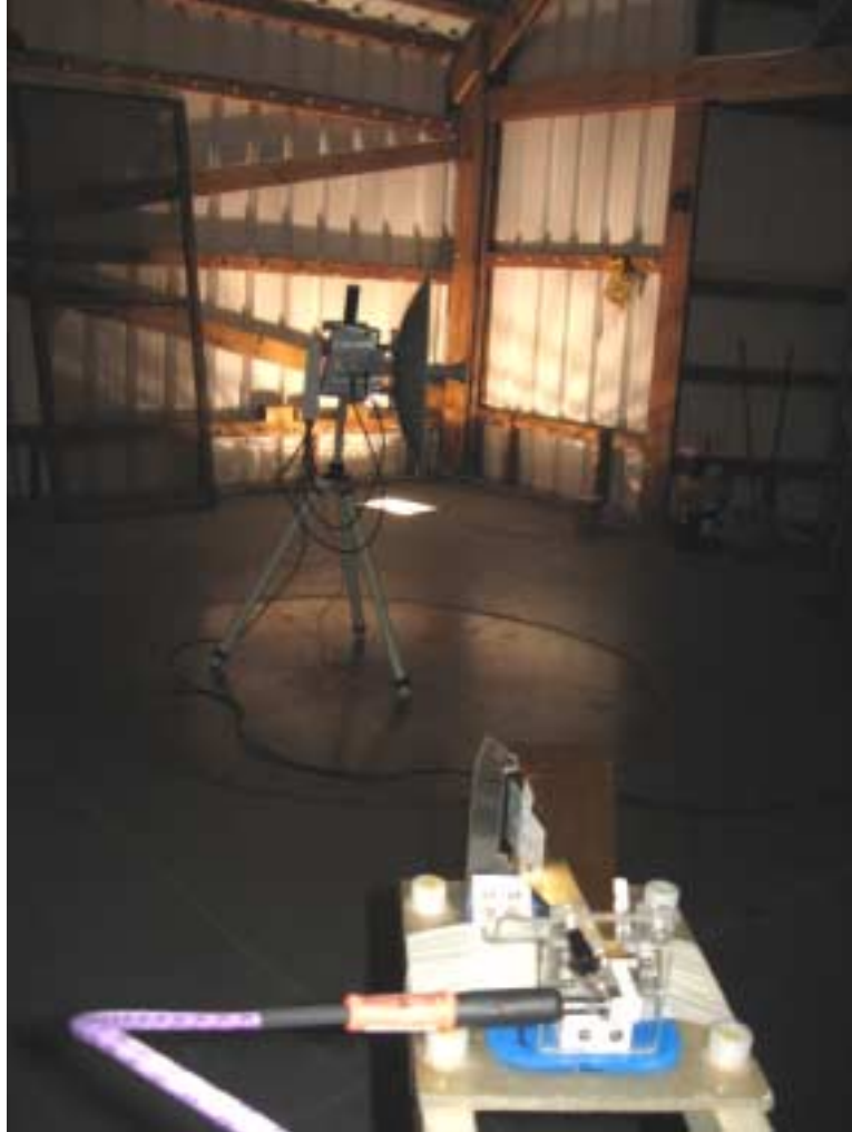
Photograph No.10 Radiated emissions measurement setup at the OATS with horn antenna, EUT with dish antenna
