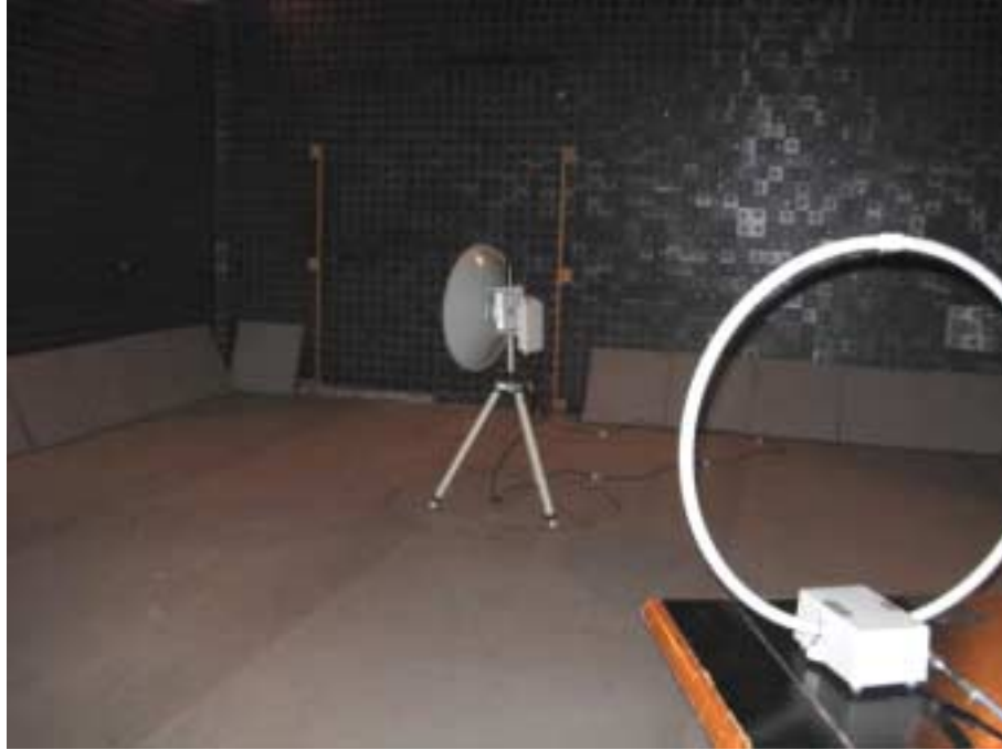
Photograph No.6 Radiated emissions measurement setup in the anechoic chamber with loop antenna, EUT with dish antenna
