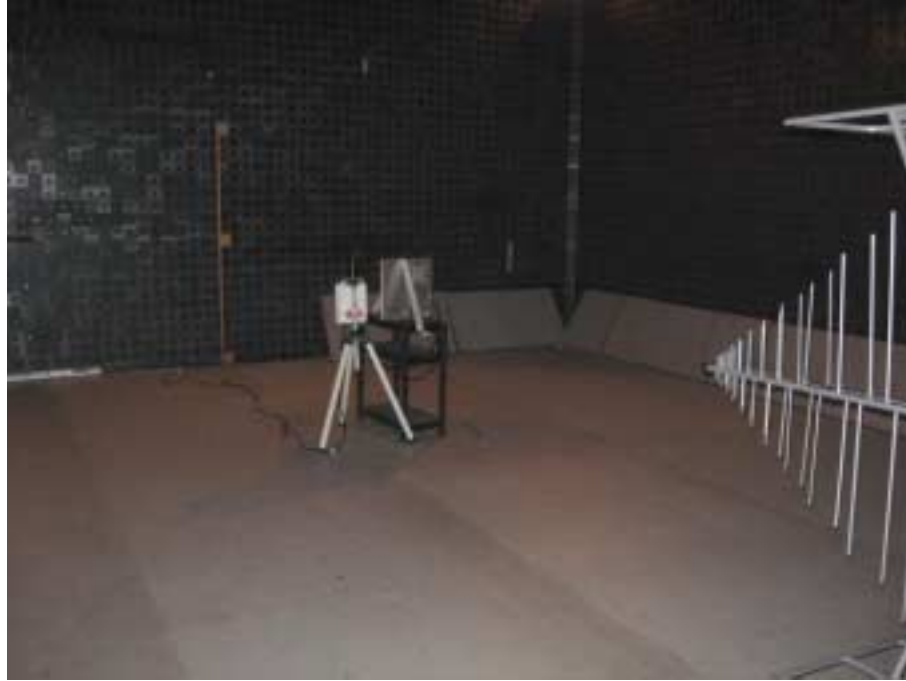
Photograph No.3 Radiated emissions measurement setup in the anechoic chamber with biconilog antenna, EUT with flat antenna
