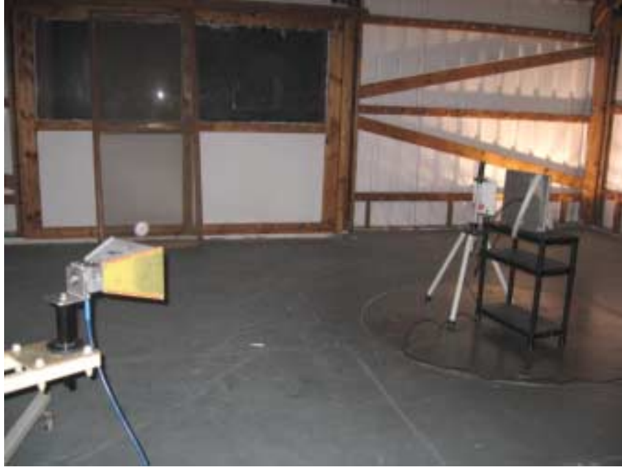
Photograph No.4 Radiated emissions measurement setup at the OATS with double ridged guide antenna, EUT with flat antenna
