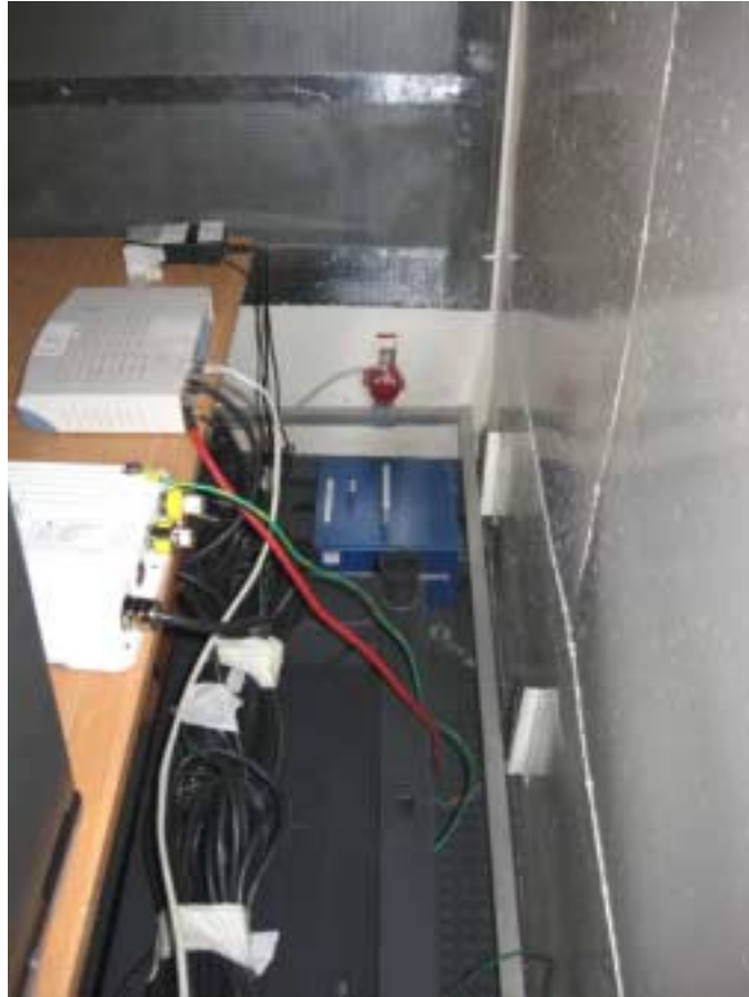
Photograph No.12 Conducted emission on power lines measurement setup
