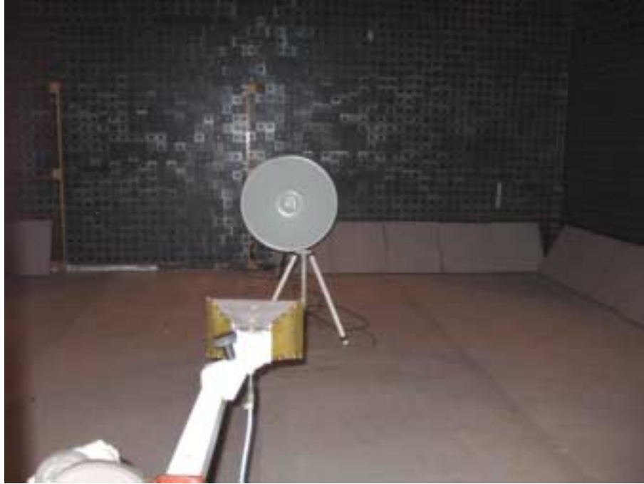
Photograph No.8 Radiated emissions measurement setup in the anechoic chamber with double ridged guide antenna, EUT with dish antenna
