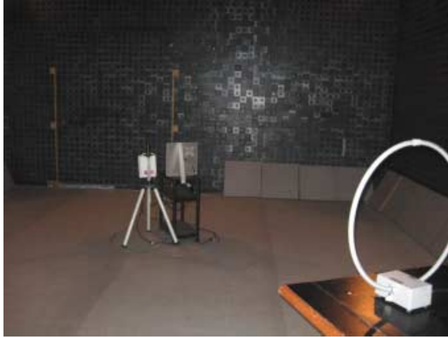
Photograph No.2 Radiated emissions measurement setup in the anechoic chamber with loop antenna, EUT with flat antenna
