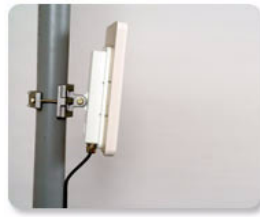
Figure 1-8: ODU with integrated Flat Panel antenna
