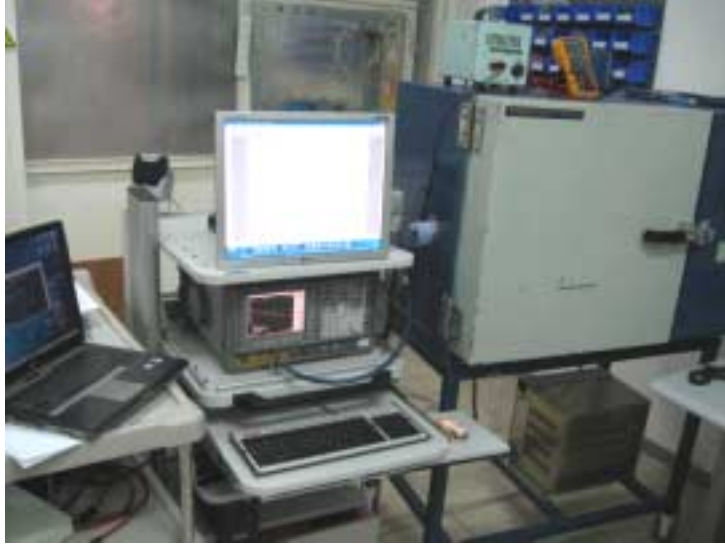
Photograph No.11 Frequency stability measurement setup
