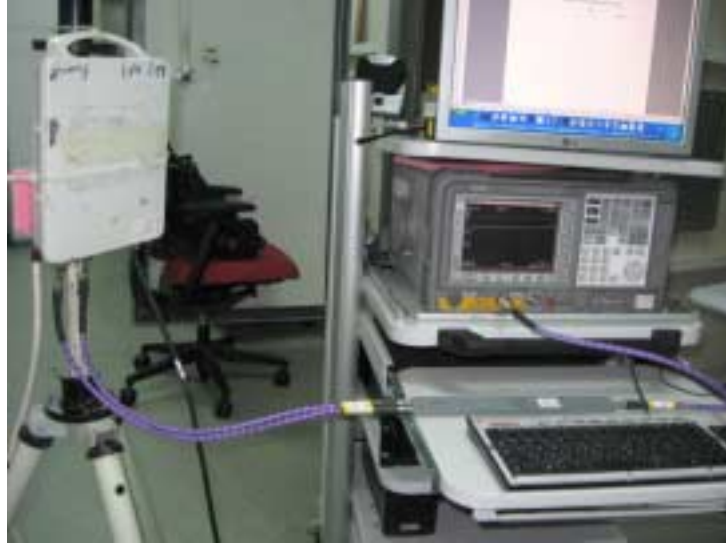
Photograph No.3 Receiver spurious emissions measurement setup
