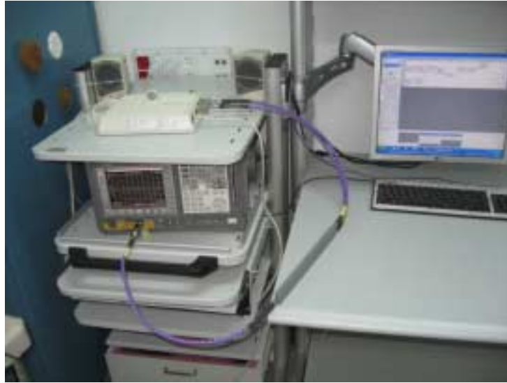
Photograph No.2 Spurious emissions measurement setup with combiner
