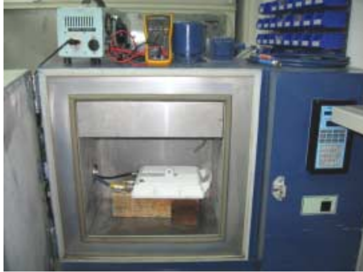
Photograph No.12 Frequency stability measurement setup
