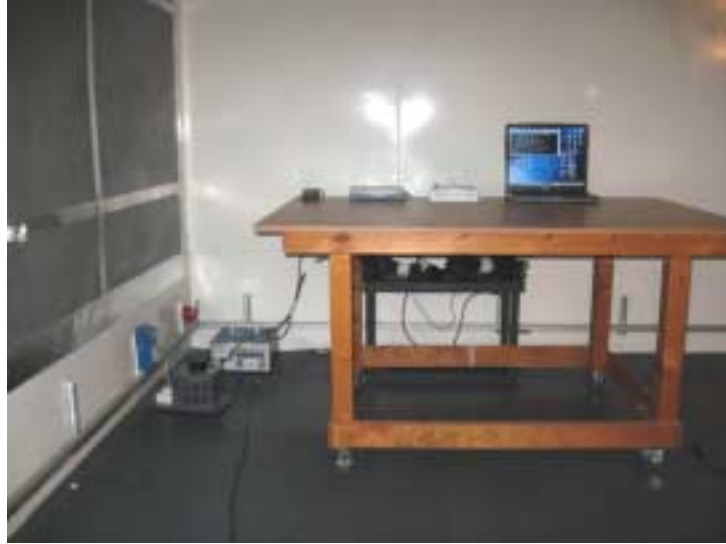
Photograph No.9 Conducted emission on power lines measurement setup
