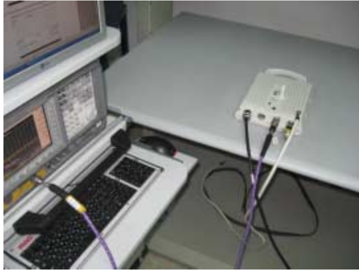
Photograph No.4 Emission mask measurement setup with combiner
