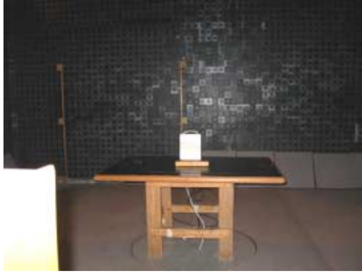
Photograph No.7 Radiated emissions measurement setup at the OATS with double ridged guide antenna
