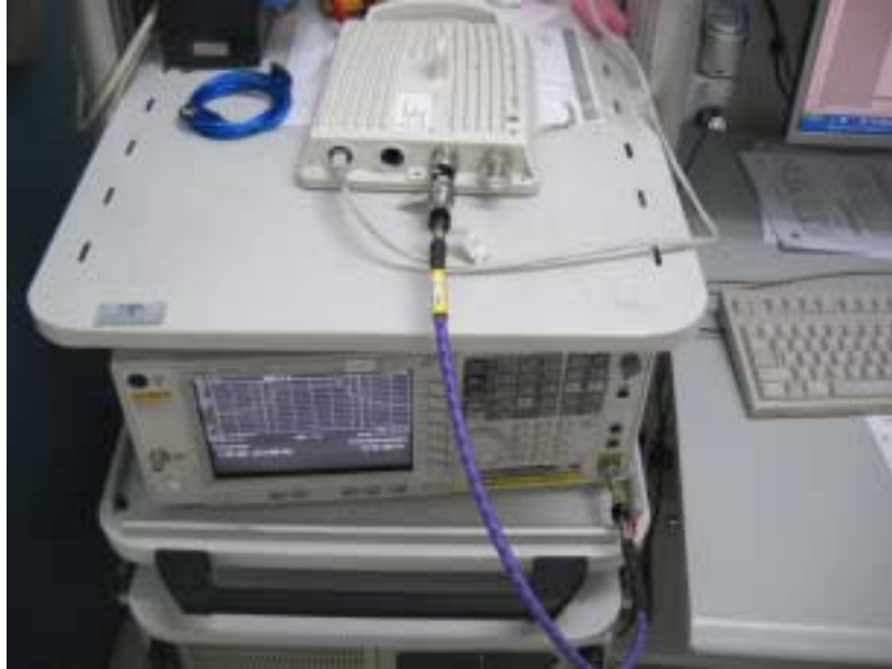
Photograph No.1 Peak output power, peak power density, occupied bandwidth, individual RF output measurement setup
