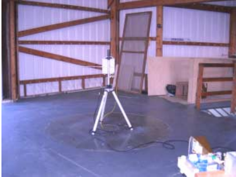
Photograph No.6 Radiated emissions measurement setup at the OATS with double ridged guide antenna
