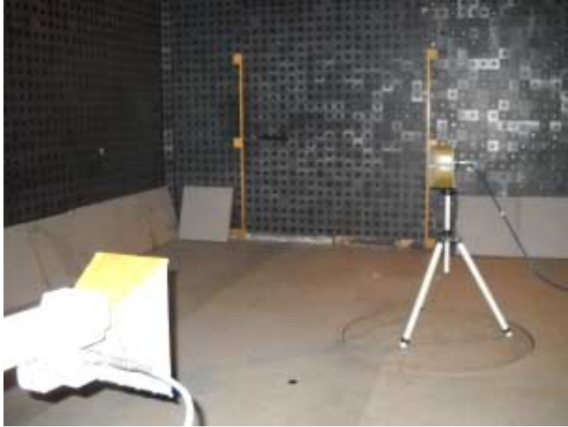
Photograph No.7 Setup for substitution ERP measurements of spurious
