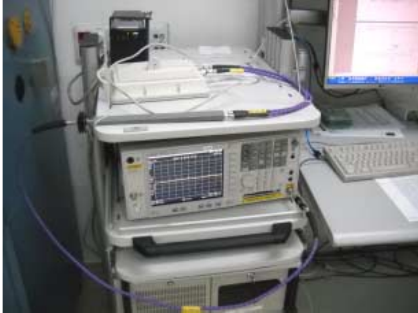
Photograph No.2 Spurious emissions measurement setup, combined RF outputs testing
