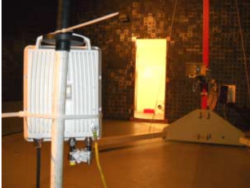
Photograph No.5 Radiated emissions measurement setup in the anechoic chamber with double ridged guide antenna
