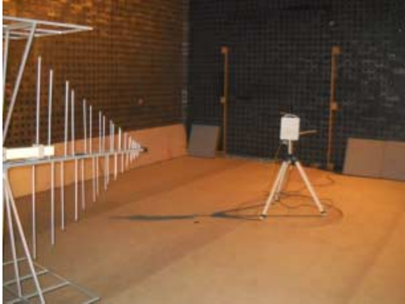
Photograph No.4 Radiated emissions measurement setup in the anechoic chamber with biconilog antenna
