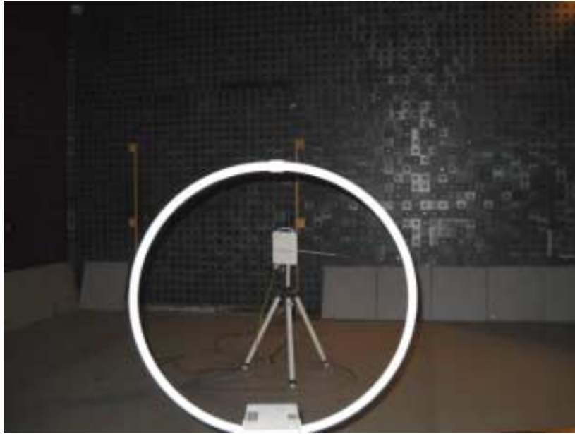
Photograph No.3 Radiated emissions measurement setup in the anechoic chamber with loop antenna
