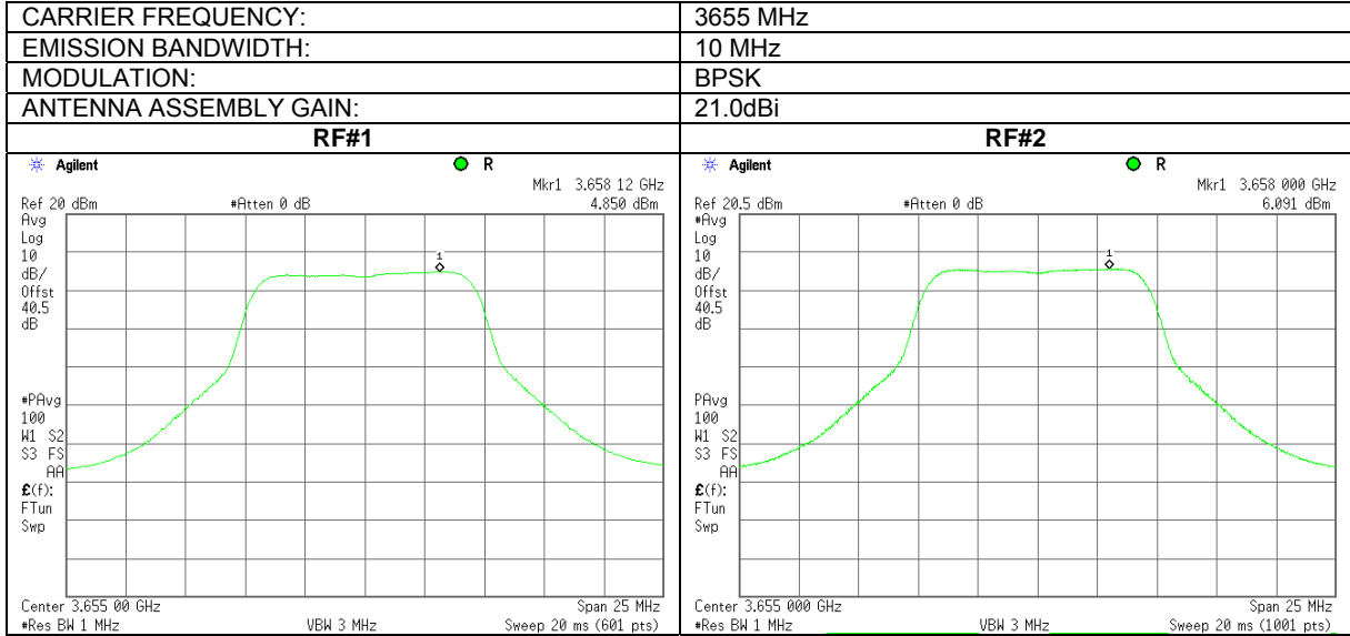
Plot 7.2.8 Peak output power density test results at low frequency
