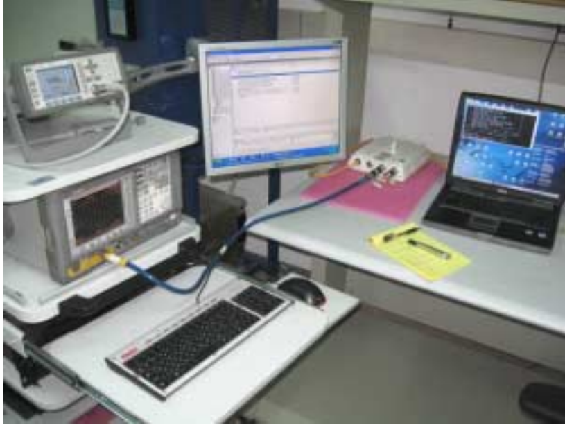
Photograph No.5 Peak spectral power density measurement setup
