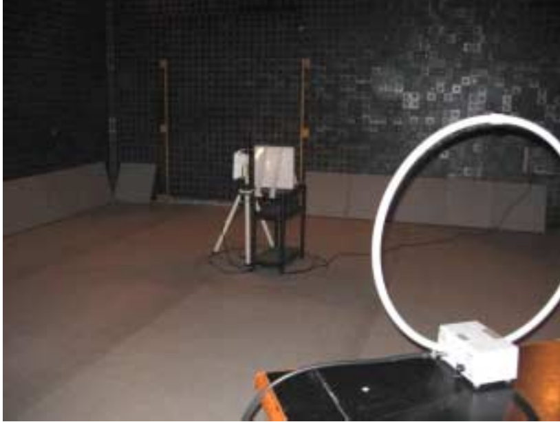
Photograph No.5 Radiated emissions measurement setup in the anechoic chamber with loop antenna
