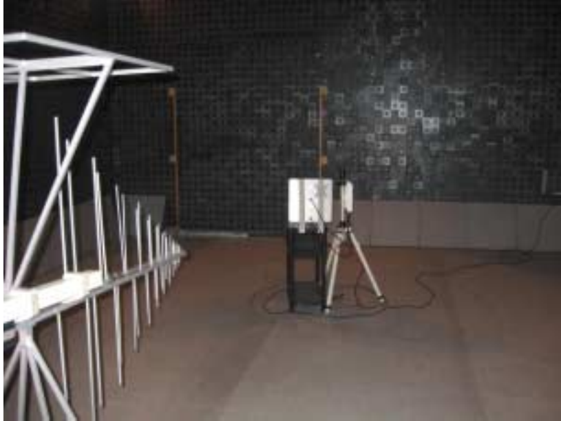
Photograph No.6 Radiated emissions measurement setup in the anechoic chamber with biconilog antenna
