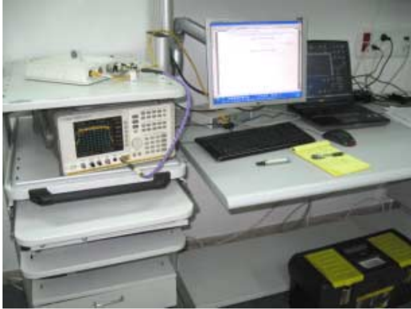
Photograph No.2 Occupied bandwidth measurement setup
