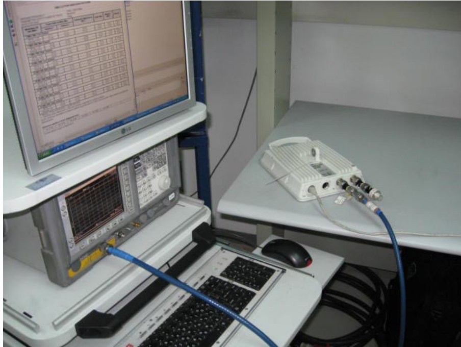
Photograph No.3 Spurious emissions measurement setup, individual RF output testing
