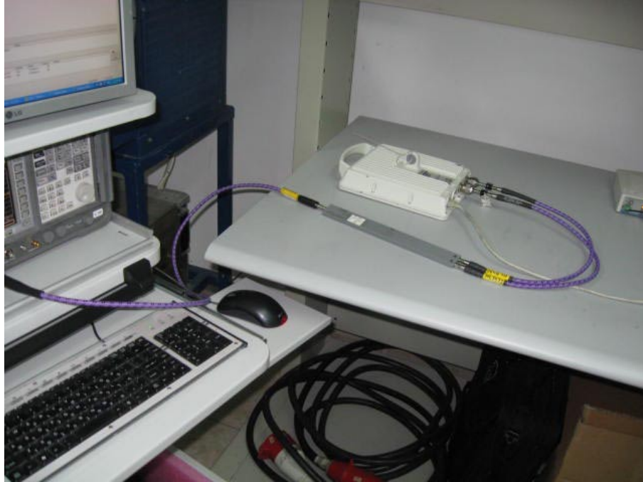
Photograph No.4 Spurious emissions measurement setup, combined RF outputs testing
