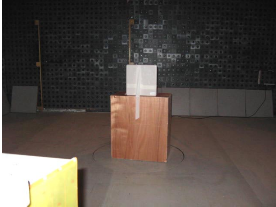
Photograph No.7 Radiated emissions measurement setup in the anechoic chamber with double ridged guide antenna
