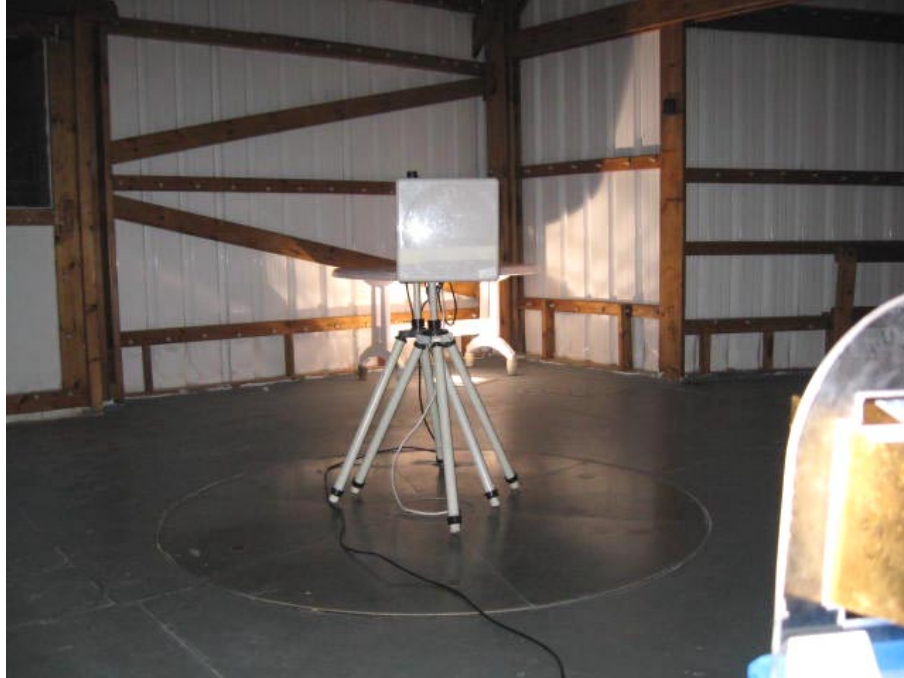
Photograph No.9 Radiated emissions measurement setup at the OATS with horn antenna
