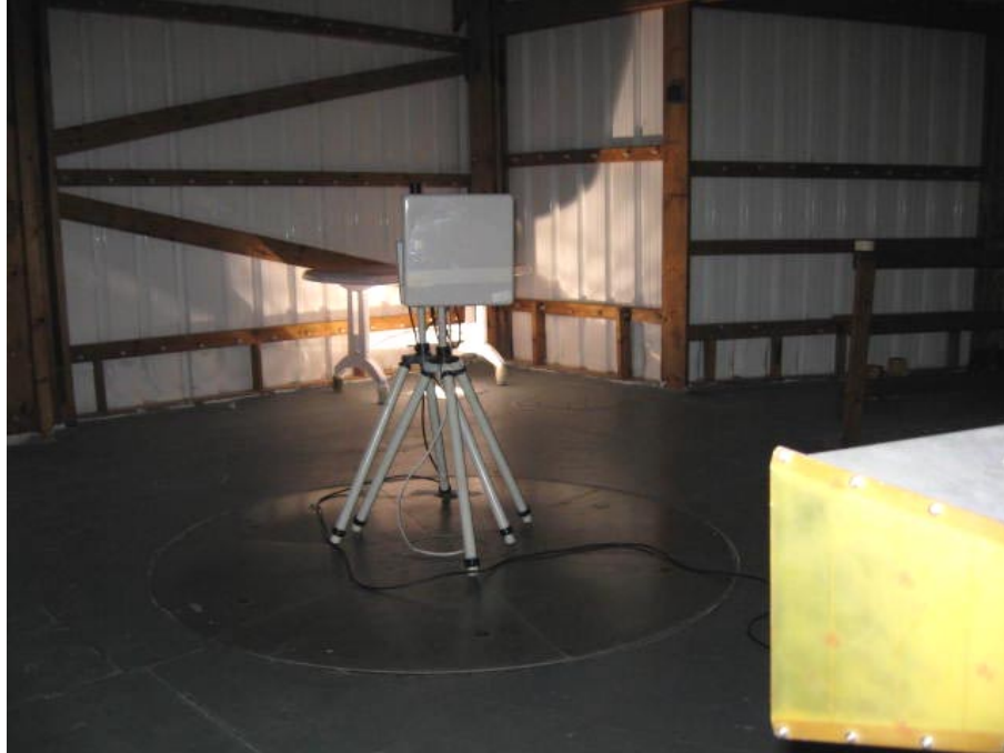
Photograph No.8 Radiated emissions measurement setup at the OATS with double ridged guide antenna
