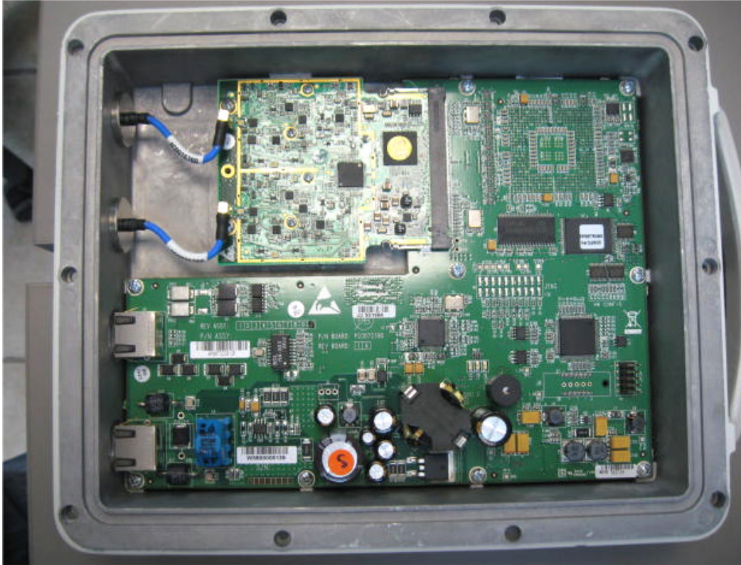
Photograph No2 RADWIN 2000 internal view
