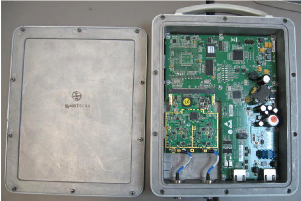
Photograph No.1 RADWIN 2000 internal view with cover removed
