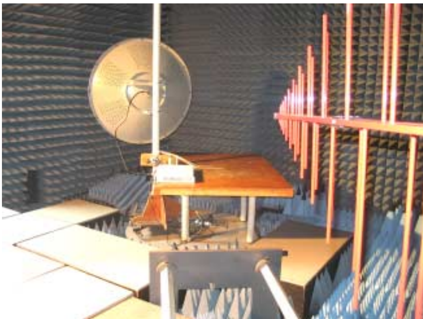
Photograph No.11 Radiated emissions measurement setup in the anechoic chamber with biconilog antenna EUT: AIND with 32.5 dBi antenna
