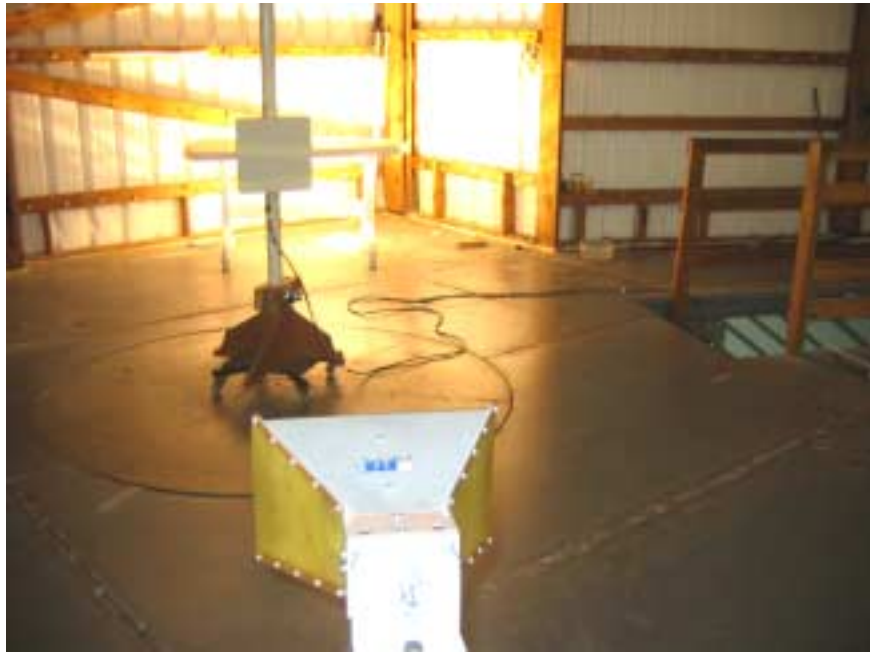
Photograph No.14 Radiated emissions measurement setup at the OATS with double ridged guide antenna EUT: ODU with 22 dBi antenna
