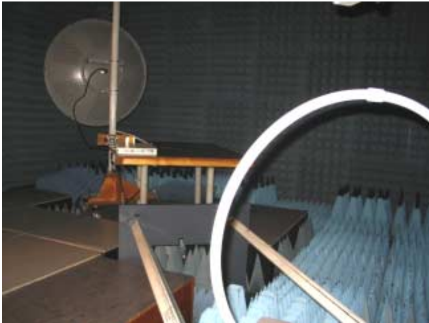
Photograph No.6 Radiated emissions measurement setup in the anechoic chamber with loop antenna EUT: AIND with 32.5 dBi antenna
