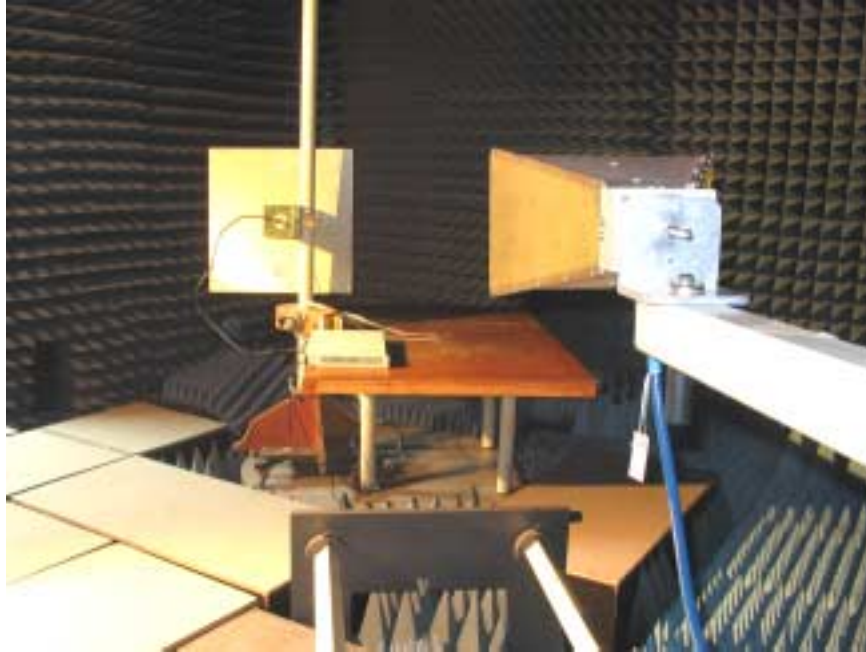
Photograph No.12 Radiated emissions measurement setup in the anechoic chamber with double ridged guide antenna EUT: AIND with 28 dBi antenna
