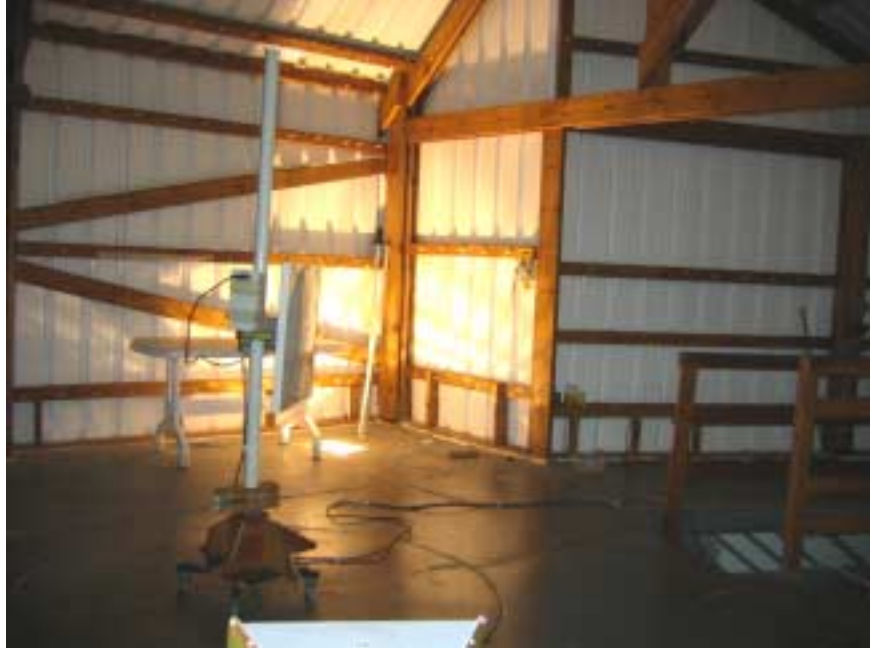
Photograph No.15 Radiated emissions measurement setup at the OATS with double ridged guide antenna EUT: ODU with 28 dBi antenna
