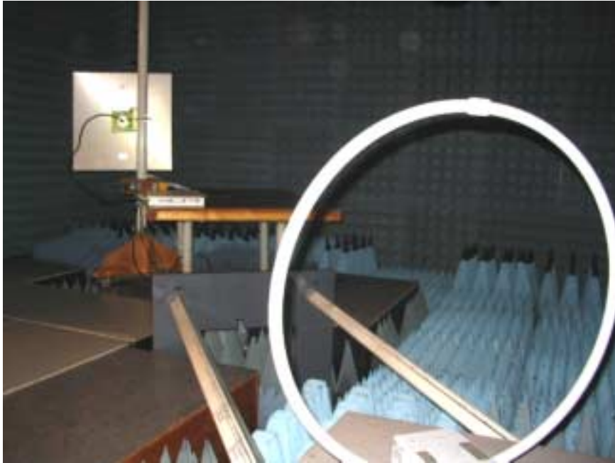
Photograph No.5 Radiated emissions measurement setup in the anechoic chamber with loop antenna EUT: AIND with 28 dBi antenna
