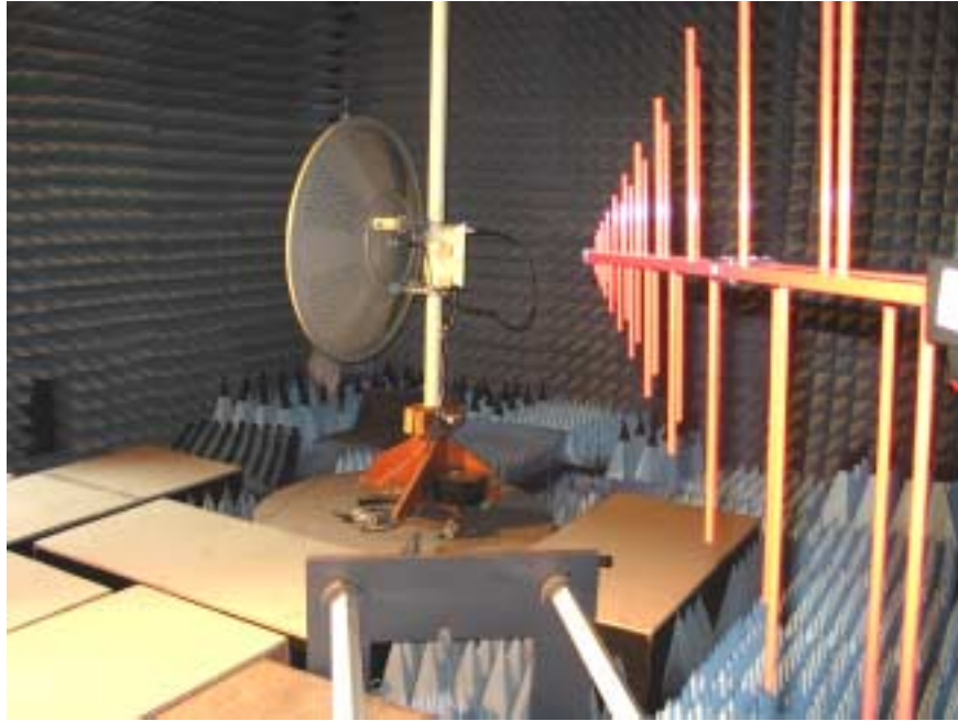
Photograph No.7 Radiated emissions measurement setup in the anechoic chamber with biconilog antenna EUT: ODU with 32.5 dBi antenna
