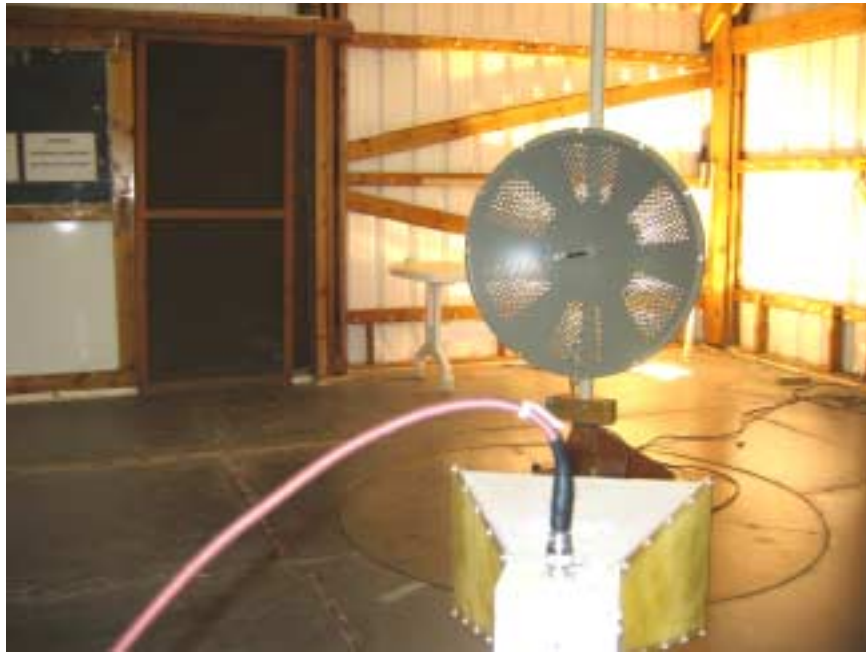
Photograph No.17 Radiated emissions measurement setup at the OATS with double ridged guide antenna EUT: AIND with 32.5 dBi antenna
