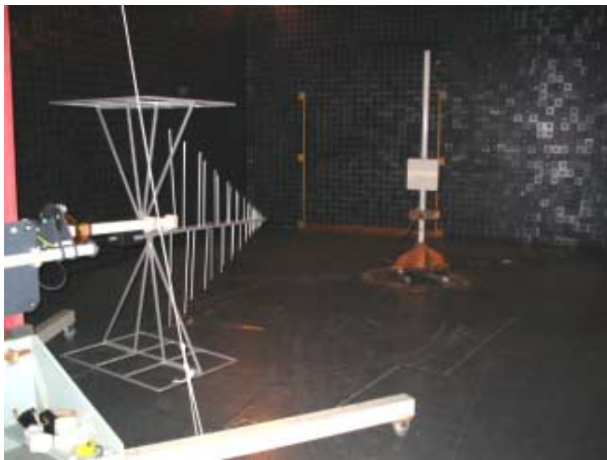
Photograph No.8 Radiated emissions measurement setup in the anechoic chamber with biconilog antenna EUT: ODU with 22 dBi antenna
