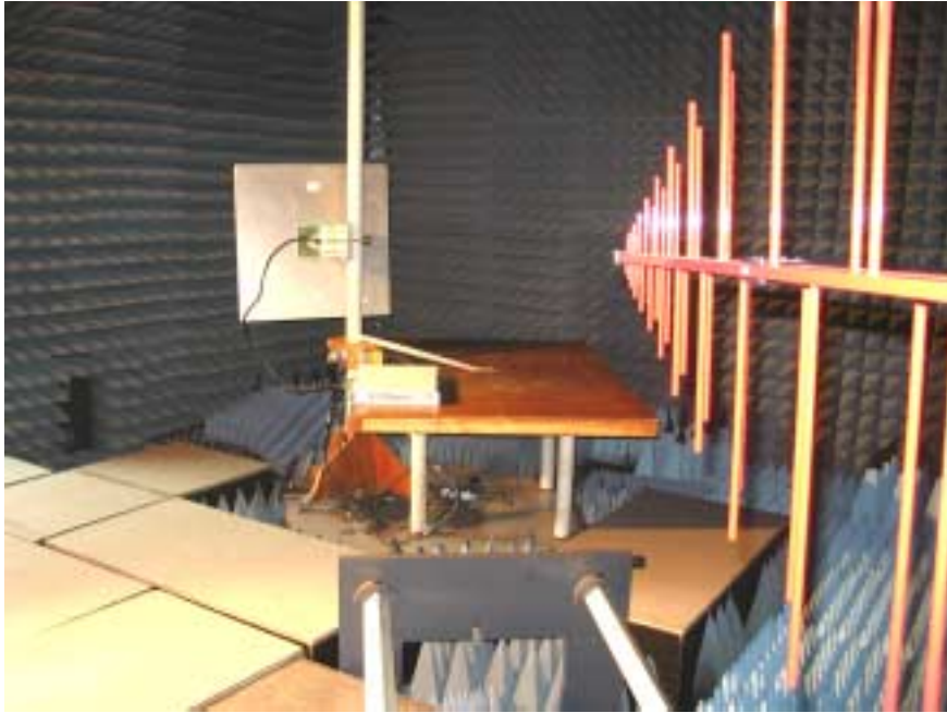
Photograph No.11 Radiated emissions measurement setup in the anechoic chamber with biconilog antenna EUT: AIND with 32.5 dBi antenna
