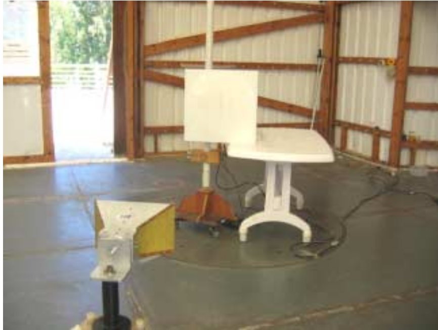
Photograph No.16 Radiated emissions measurement setup at the OATS with double ridged guide antenna EUT: AIND with 28 dBi antenna
