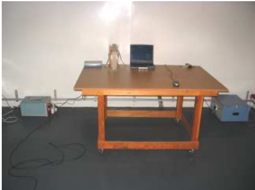
Photograph No.19 Conducted emissions measurement setup on ODU power lines
