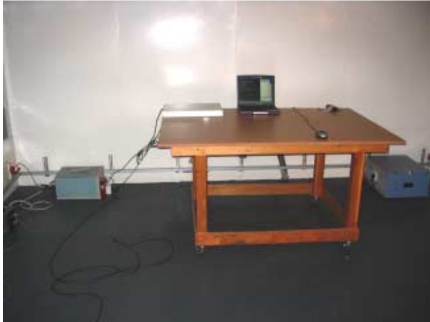
Photograph No.18 Conducted emissions measurement setup on AIND power lines
