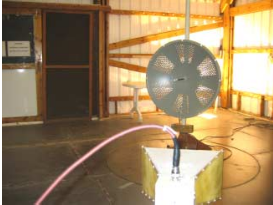
Photograph No.13 Radiated emissions measurement setup at the OATS with double ridged guide antenna EUT: ODU with 32.5 dBi antenna
