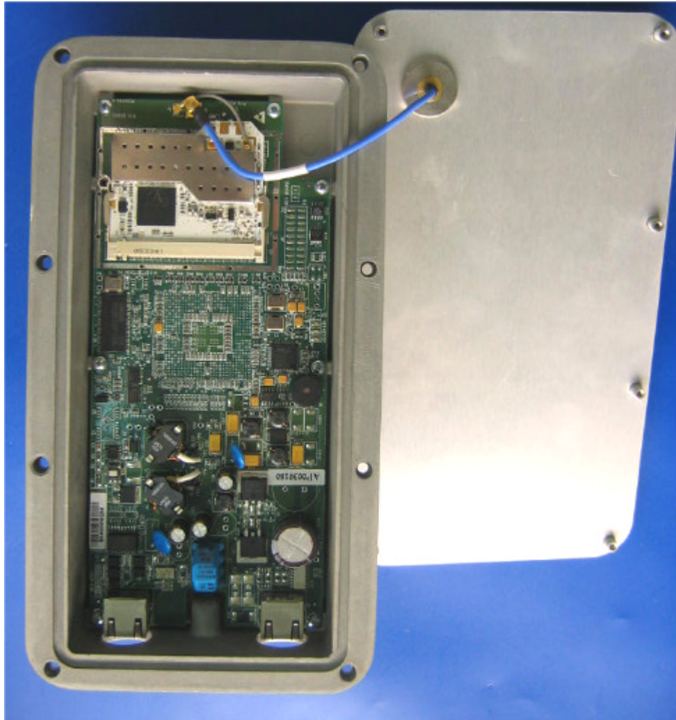
Photograph No.9 Winlink 1000-F58/HP (ODU) internal view
