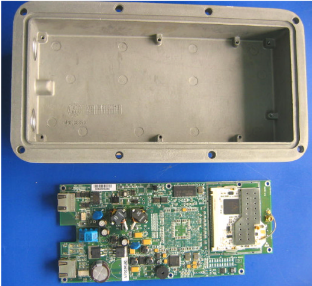
Photograph No.11 Winlink 1000-F58/HP (ODU)internal view, PCB removed from the case
