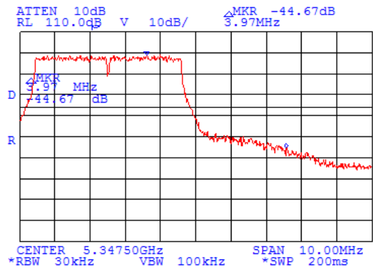
Plot 7.3.17 Radiated emission measurements at high edge by delta method
