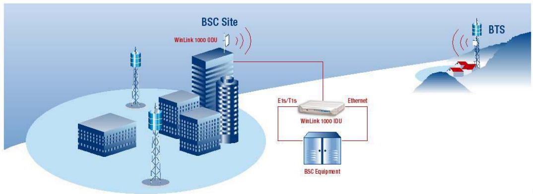
Figure 1-1: Typical Cellular Backhaul Application
