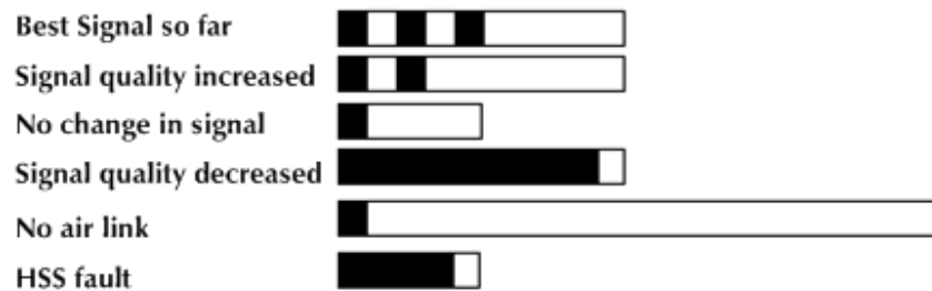
Figure 3-8: Beeper Sequence for ODU Alignment
