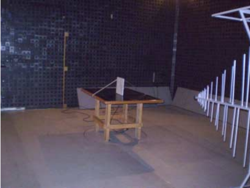
Photograph No.4 Radiated emissions measurement setup in the anechoic chamber with biconilog antenna, EUT with integral antenna
