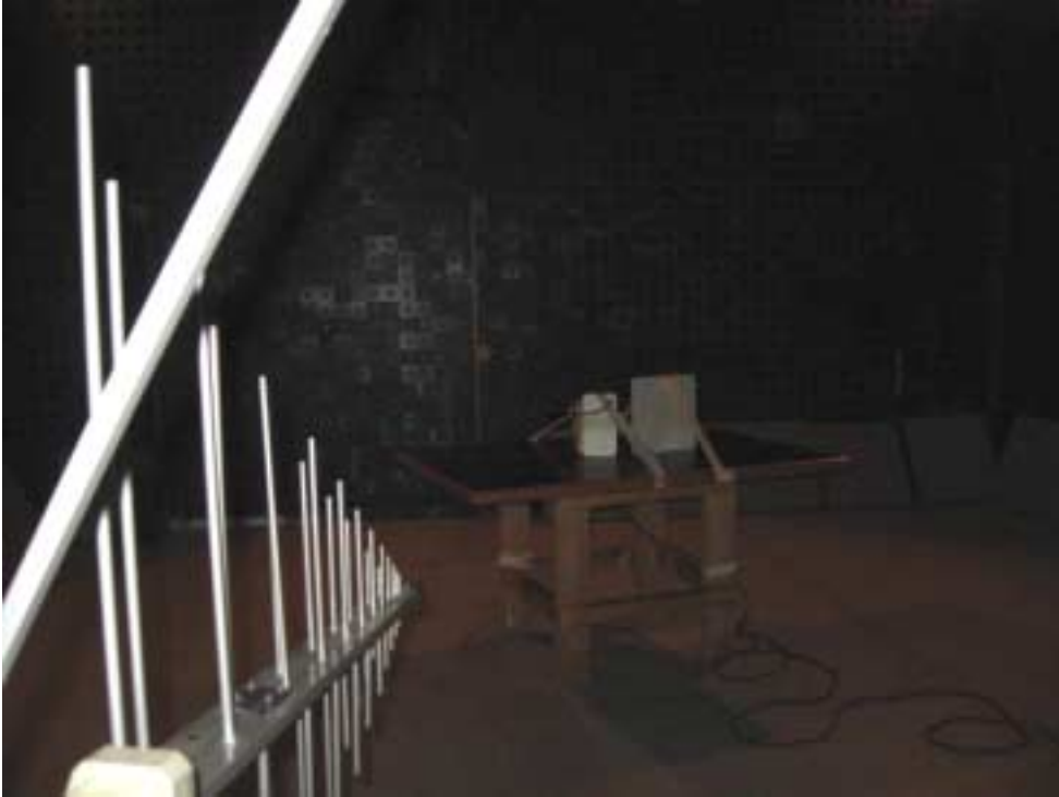
Photograph No.5 Radiated emissions measurement setup in the anechoic chamber with biconilog antenna, EUT with external antenna
