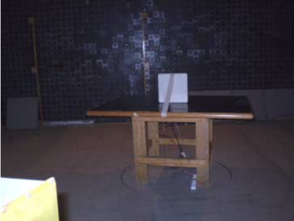
Photograph No.7 Radiated emissions measurement setup in the anechoic chamber with double ridged guide antenna, EUT with integral antenna
