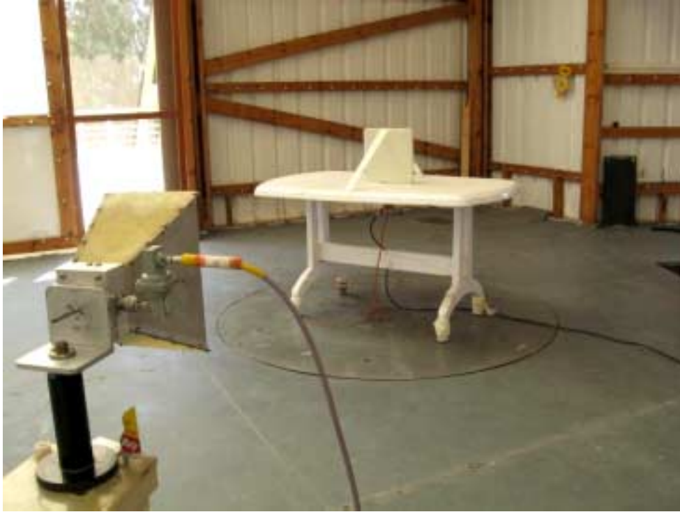
Photograph No.9 Radiated emissions measurement setup at the OATS with double ridged guide antenna, EUT with integral antenna
