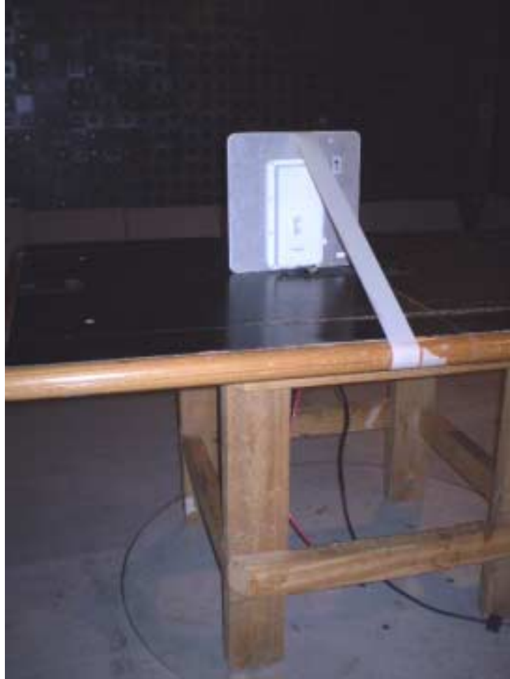
Photograph No.11 Radiated emissions measurement setup EUT with integral antenna close view
