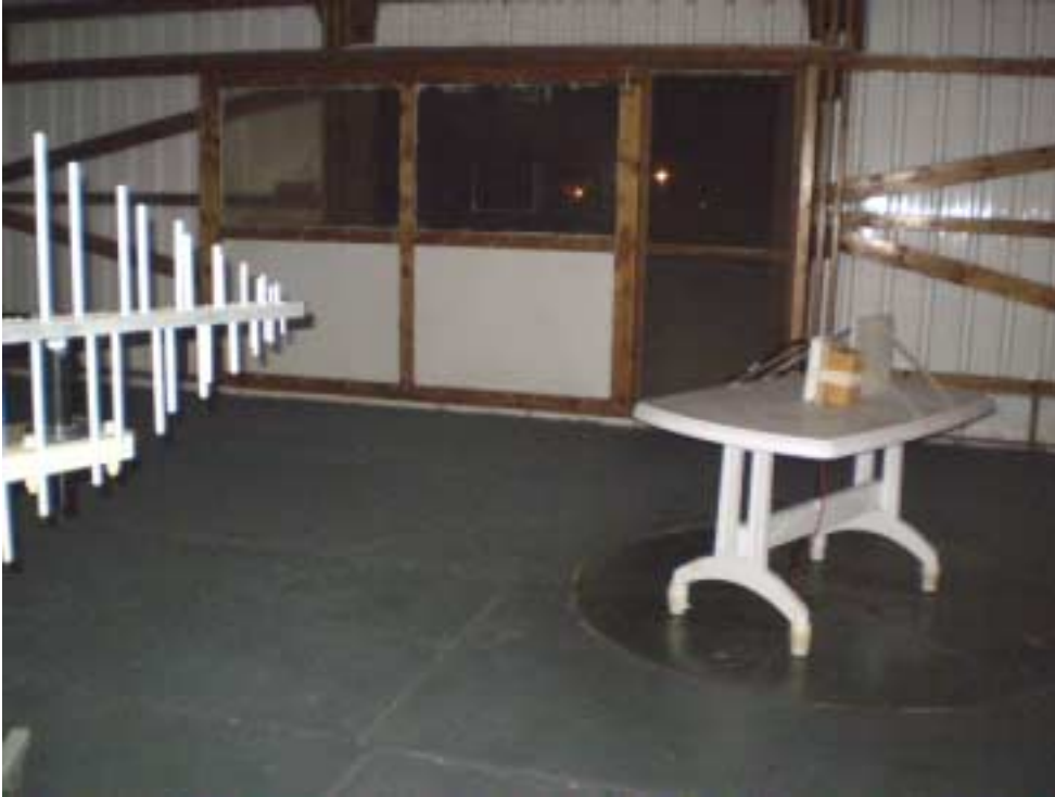
Photograph No.6 Radiated emissions measurement setup at the OATS with biconilog antenna, EUT with external antenna
