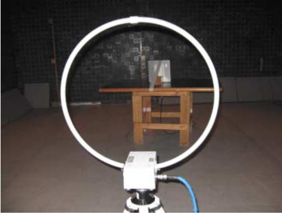
Photograph No.2 Radiated emissions measurement setup in the anechoic chamber with loop antenna, EUT with integral antenna
