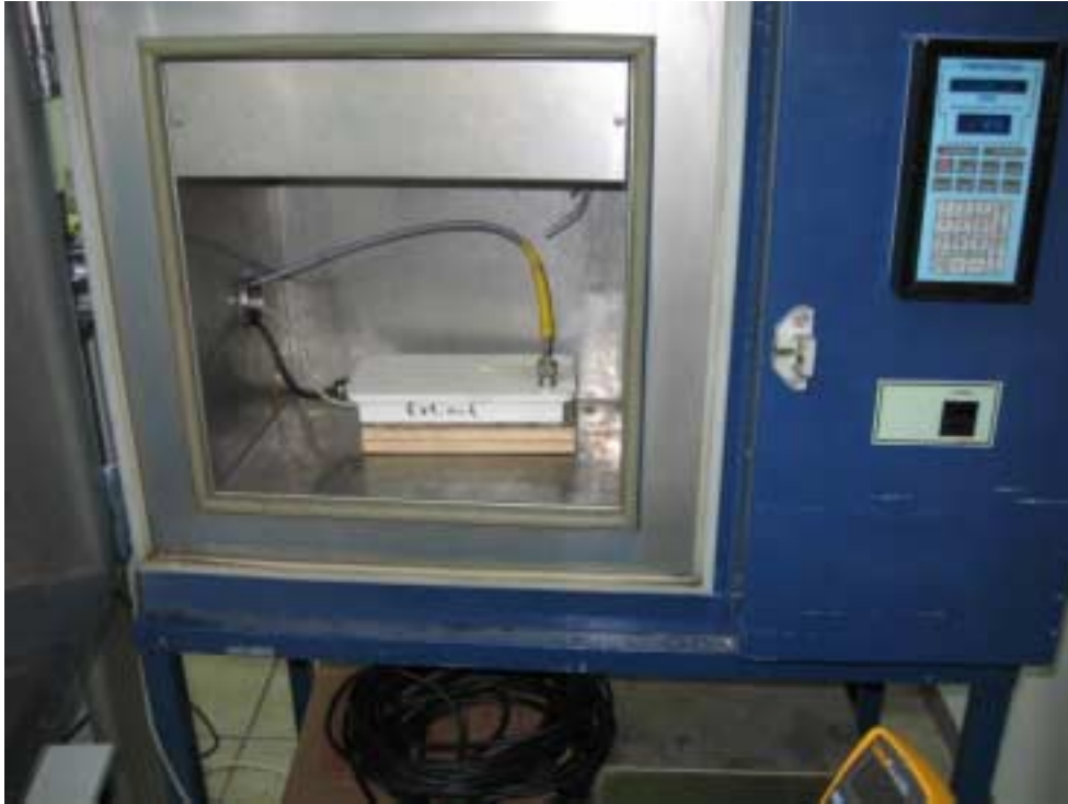
Photograph No.13 Frequency stability measurement setup
