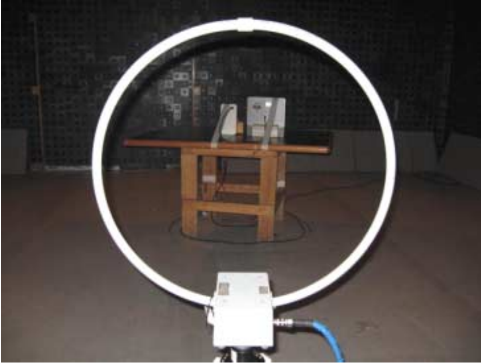
Photograph No.2 Radiated emissions measurement setup in the anechoic chamber with loop antenna, EUT with external antenna
