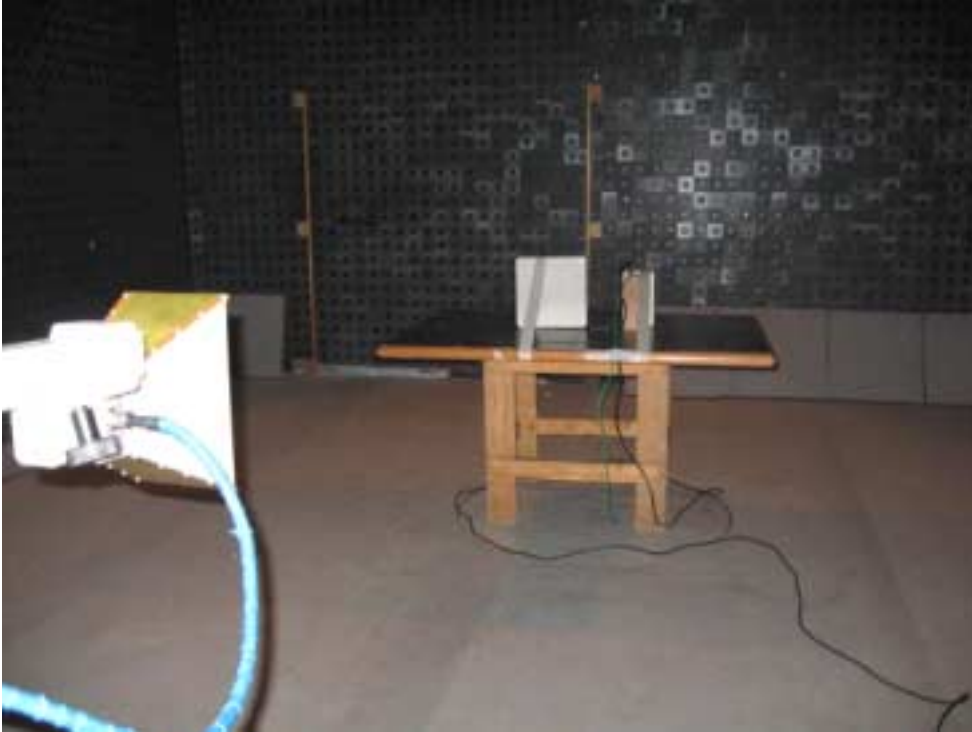
Photograph No.8 Radiated emissions measurement setup in the anechoic chamber with double ridged guide antenna, EUT with external antenna
