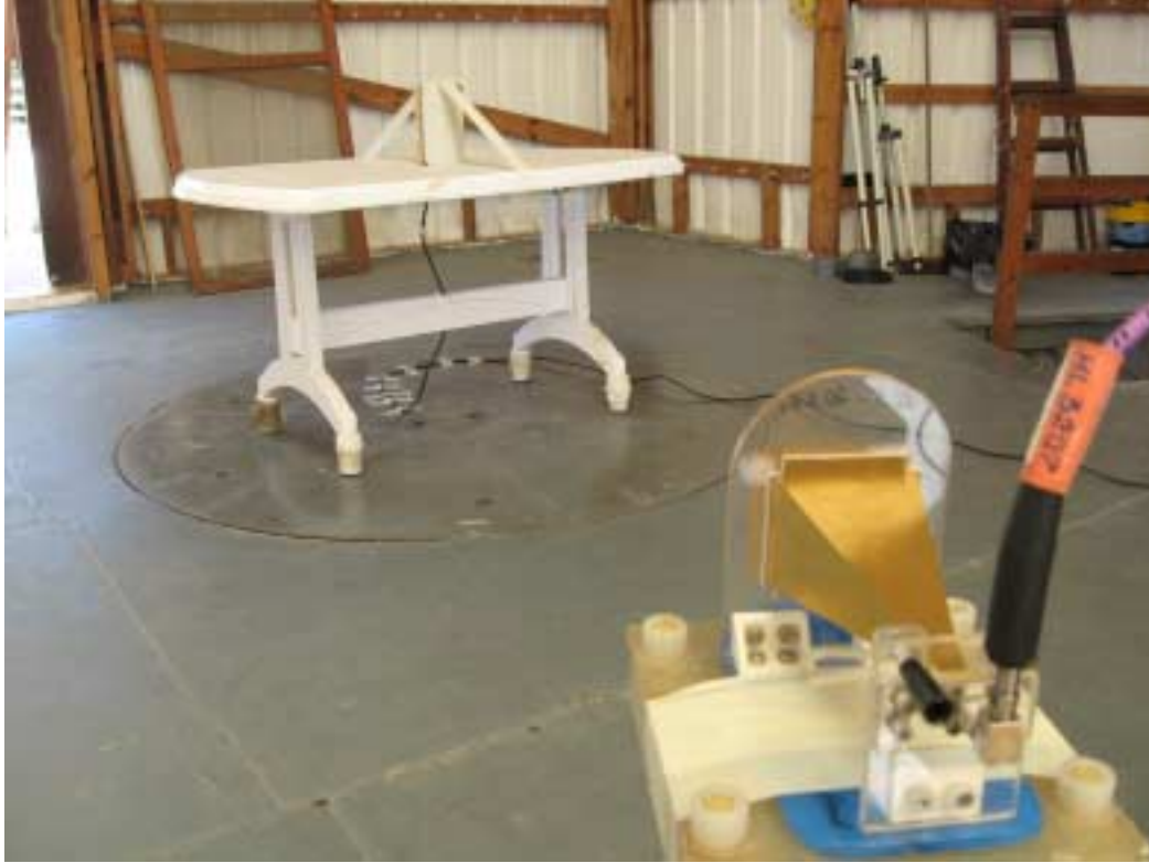
Photograph No.3 Radiated emissions measurement setup at the OATS with horn antenna
