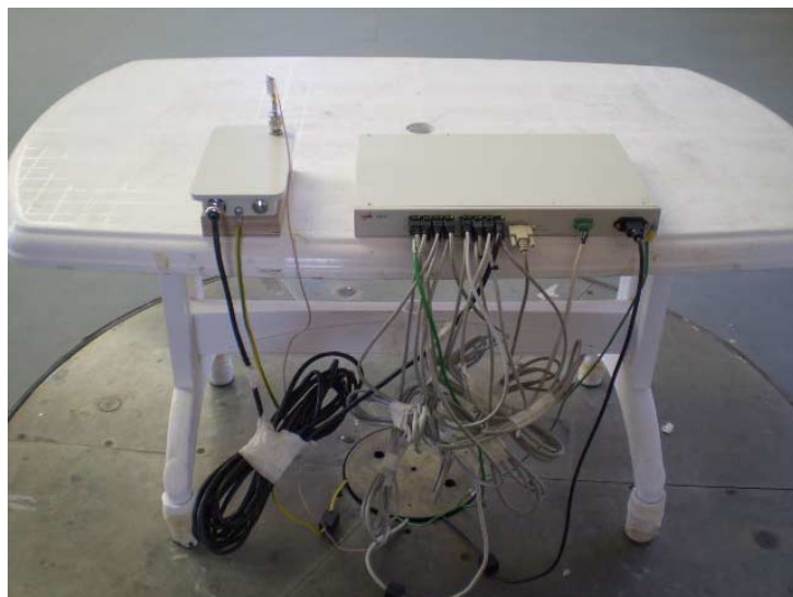
Photograph 9.1.4 Setup for radiated emission measurements at OATS, EUT cabling EUT model ODU/F24
