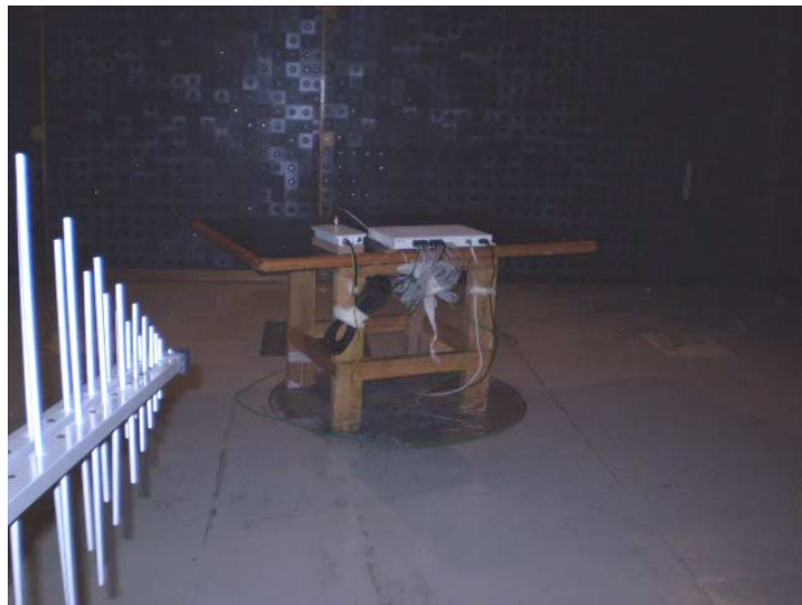
Photograph 7.1.1 Setup for radiated emission measurements in semi anechoic chamber below 1 GHz EUT model ODU/F24
