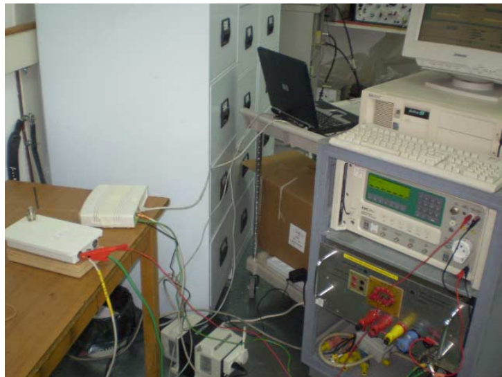
Photograph 10.4.1 Setup for conducted immunity to voltage surges at ODU line
