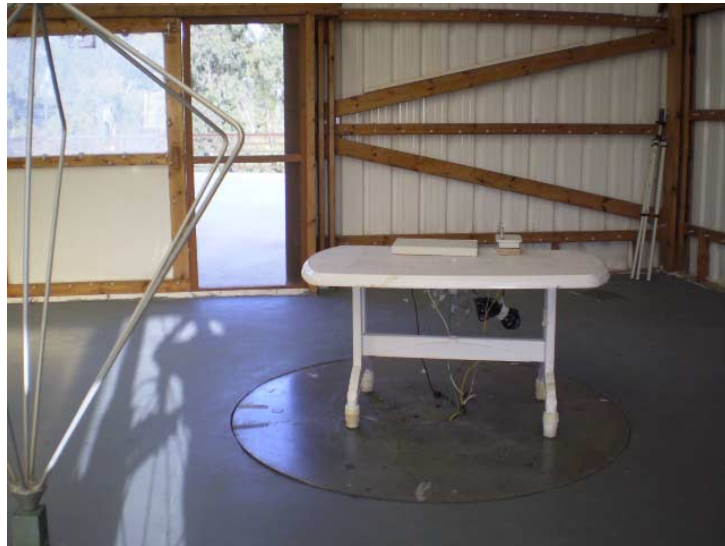
Photograph 8.1.4 Setup for radiated disturbance measurements at OATS, EUT cabling EUT model ODU/F24
