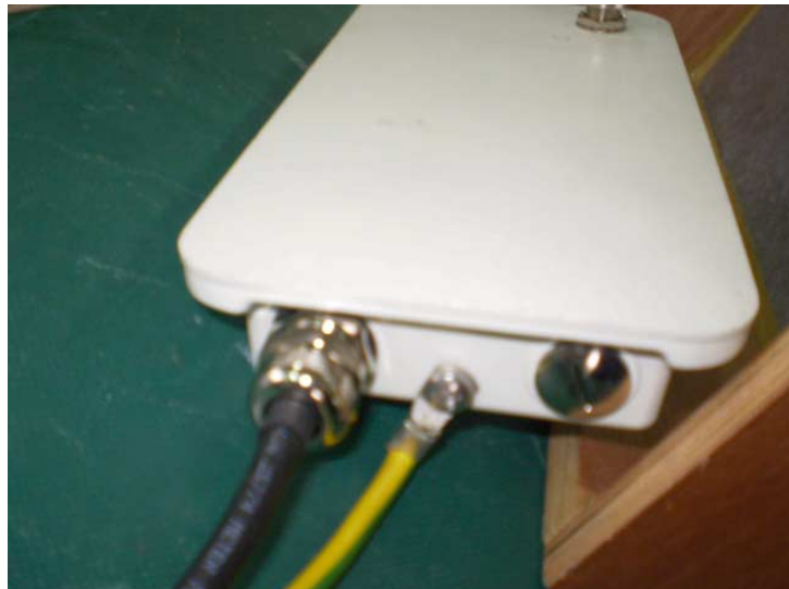
Photograph 10.1.2 Setup for immunity to ESD, EUT test points
