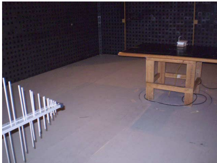
Photograph 8.1.2 Setup for radiated disturbance measurements in semi anechoic chamber EUT model ODU/F58
