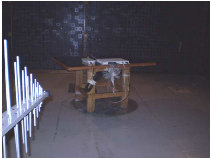
Photograph 9.1.2 Setup for radiated emission measurements in semi anechoic chamber EUT model ODU/F58
