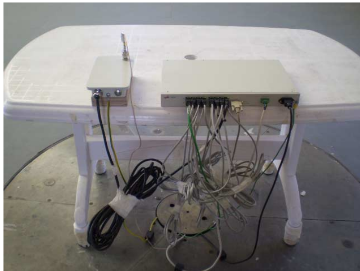
Photograph 8.1.4 Setup for radiated disturbance measurements at OATS, EUT cabling EUT model ODU/F24
