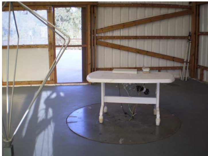
Photograph 9.1.4 Setup for radiated emission measurements at OATS, EUT cabling EUT model ODU/F24
