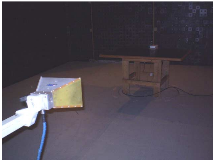
Photograph 7.1.3 Setup for radiated emission measurements in semi anechoic chamber EUT model ODU/F58
