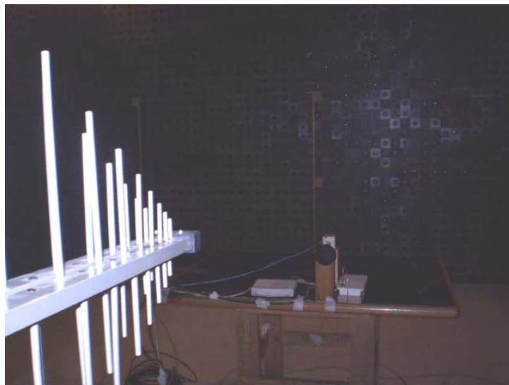
Photograph 10.2.1 Setup for radiated immunity to RF electromagnetic field test below 1 GHz, general view
