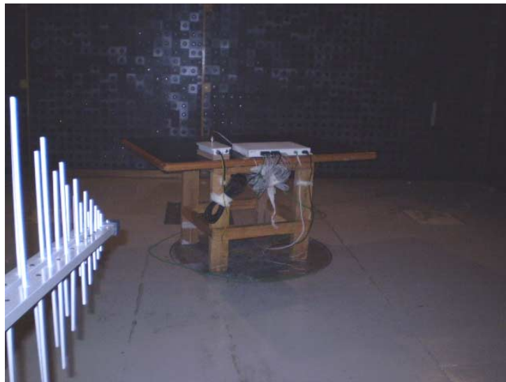
Photograph 8.1.2 Setup for radiated disturbance measurements in semi anechoic chamber EUT model ODU/F58
