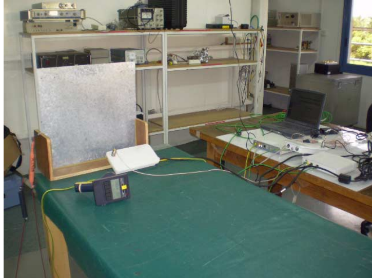
Photograph 10.1.2 Setup for immunity to ESD, EUT test points
