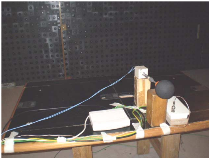
Photograph 10.2.3 Setup for radiated immunity to RF electromagnetic field test, EUT cabling
