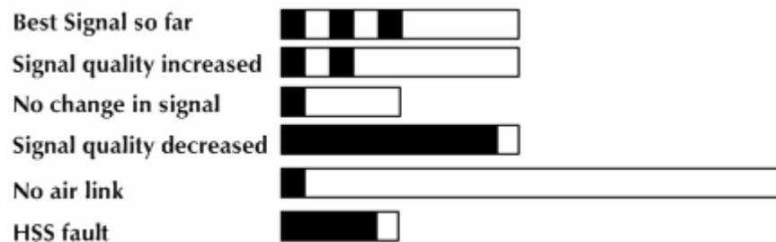
Figure 2–7. Beeper Sequence for ODU Alignment
