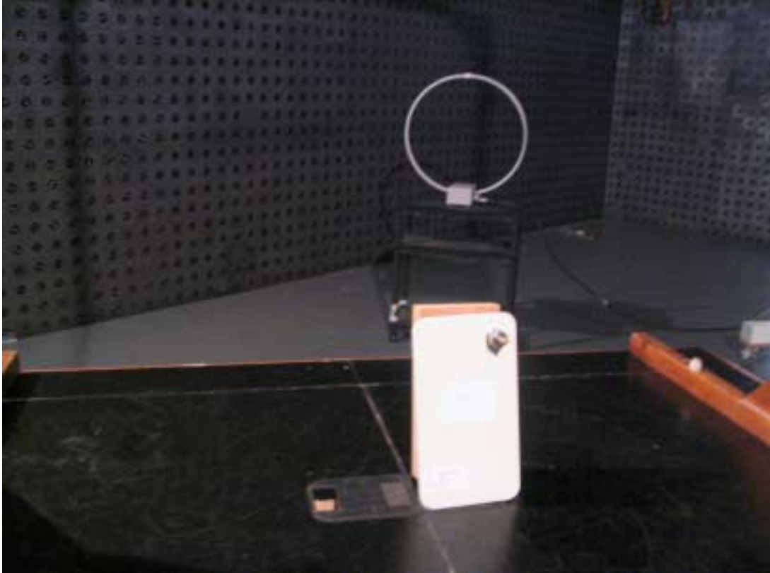
Photograph No.2 Radiated emissions measurement setup in the anechoic chamber with loop antenna
