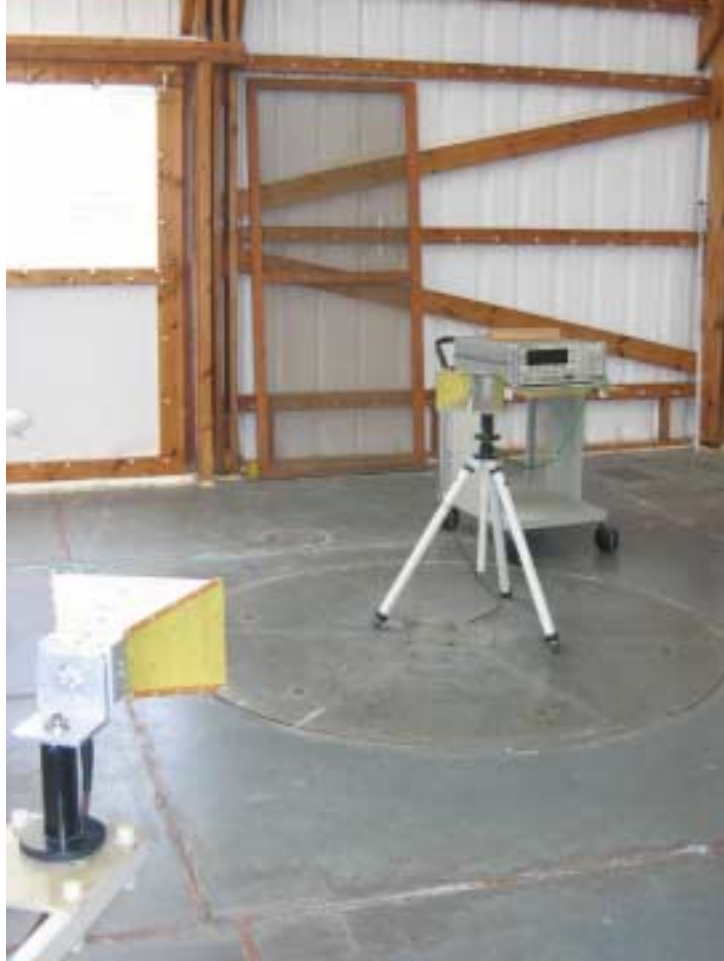
Photograph No.5 Setup for substitution ERP measurements of spurious
