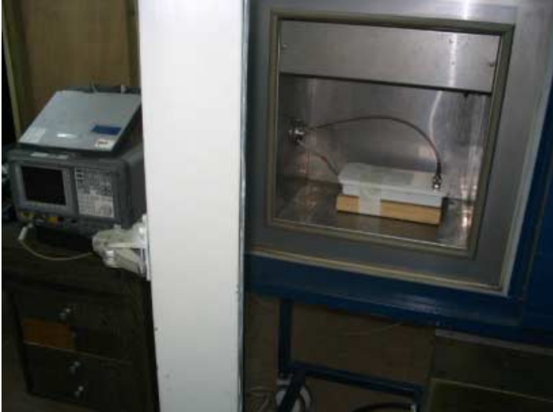
Photograph No.8 Frequency stability test setup
