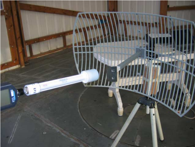
Photograph 7.3.2 Maximum permissible exposure (MPE) measurement set up, external antenna
