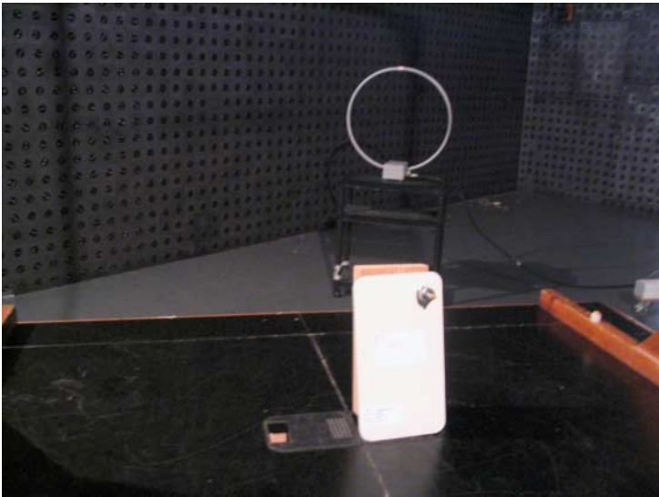
Photograph 7.7.1 Setup for spurious emission field strength measurements in 9 kHz to 30 MHz band
