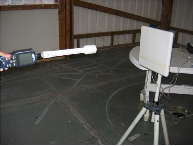
Photograph 7.3.2 Maximum permissible exposure (MPE) measurement set up, external antenna
