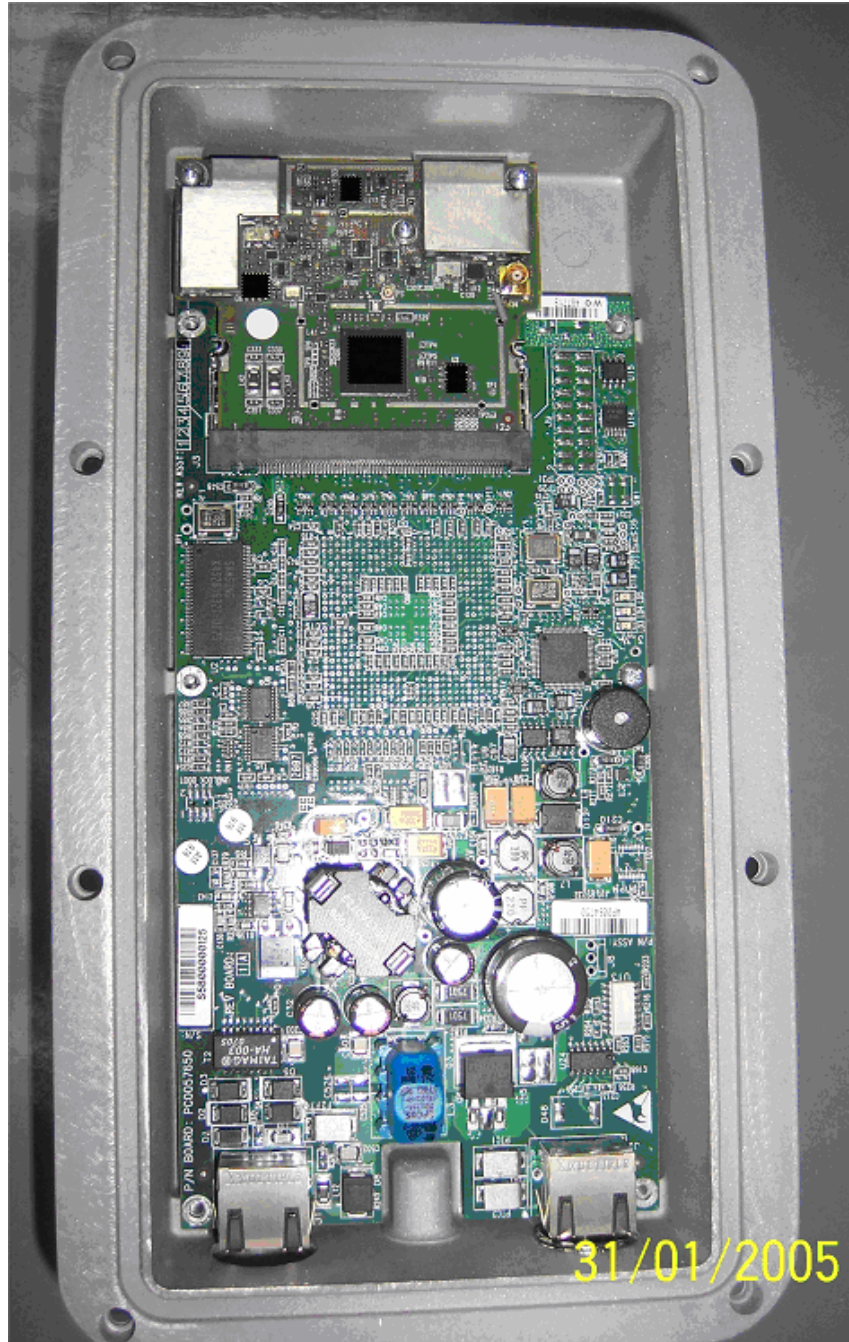
Photograph No.2 Winlink 1000-HE/F25/BRS (ODU) internal view without cover
