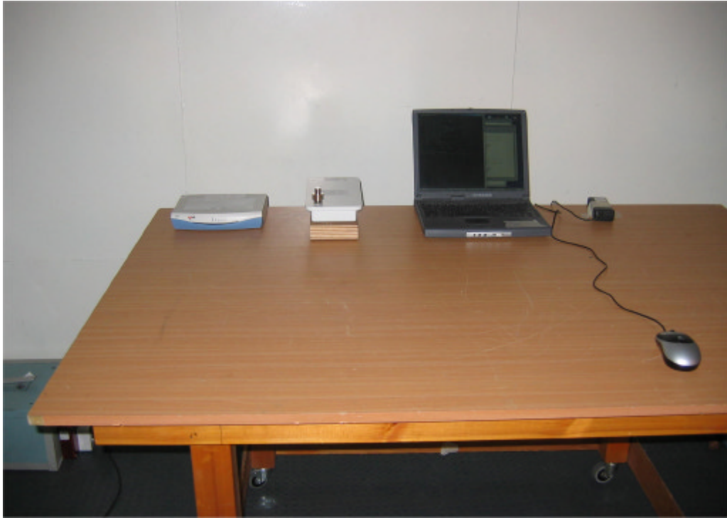
Conducted emissions measurement setup on power lines, EUT close view
