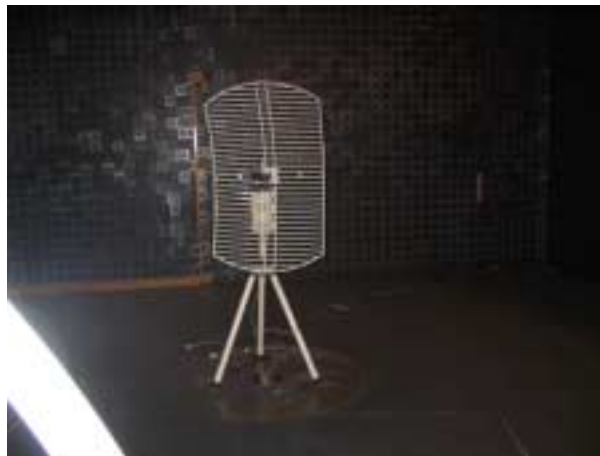
Photograph 7.5.1 Setup for spurious emission field strength measurements below 30 MHz
