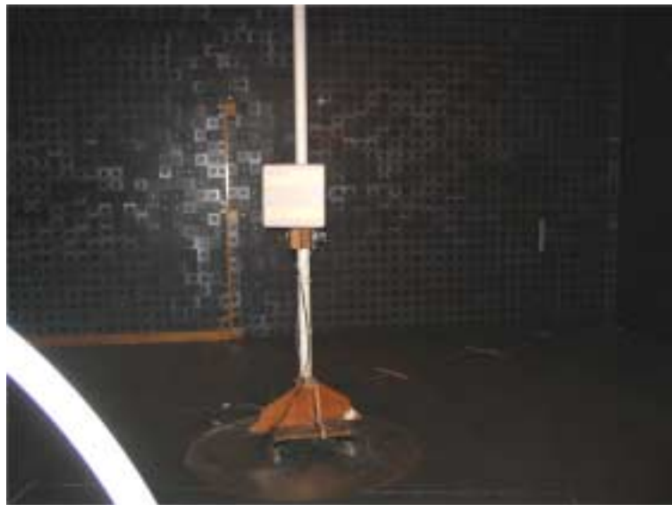
Photograph 7.4.1 Setup for spurious emission field strength measurements below 30 MHz
