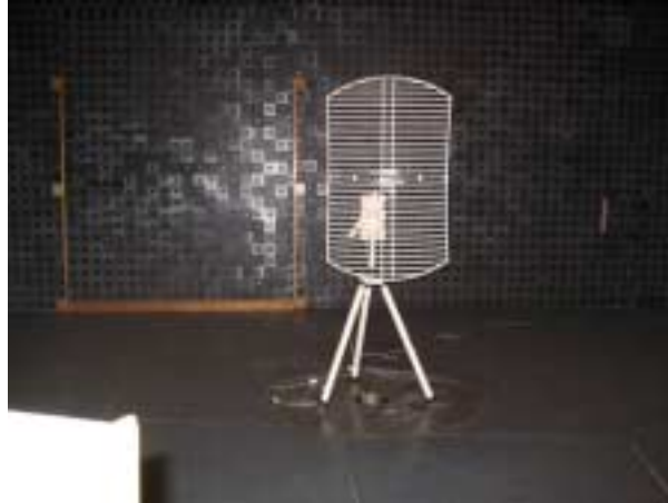
Photograph 7.5.3 Setup for spurious emission field strength measurements above 1000 MHz
