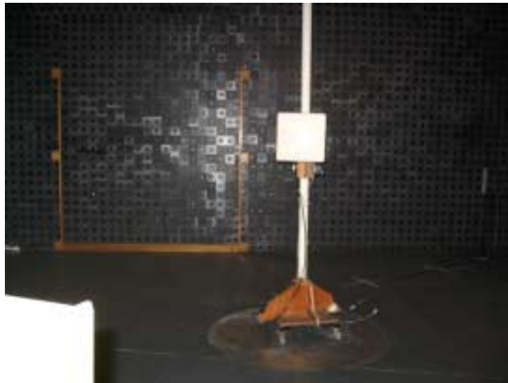
Photograph 7.4.3 Setup for spurious emission field strength measurements above 1000 MHz
