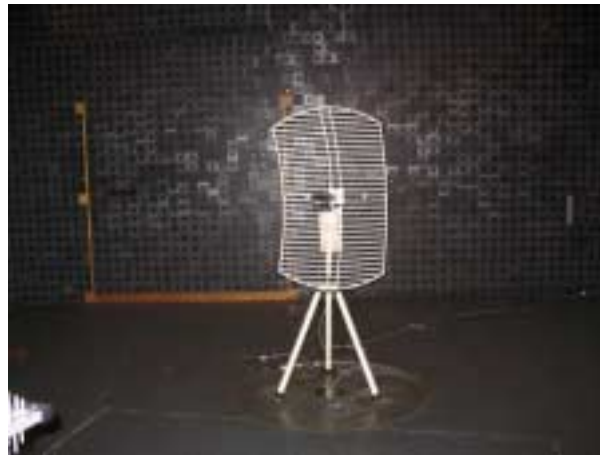
Photograph 7.5.2 Setup for spurious emission field strength measurements from 30 to 1000 MHz
