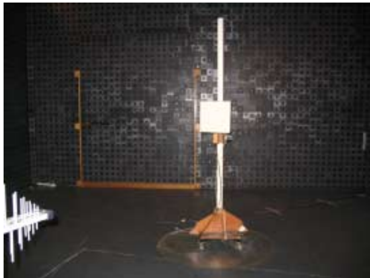
Photograph 7.4.2 Setup for spurious emission field strength measurements from 30 to 1000 MHz
