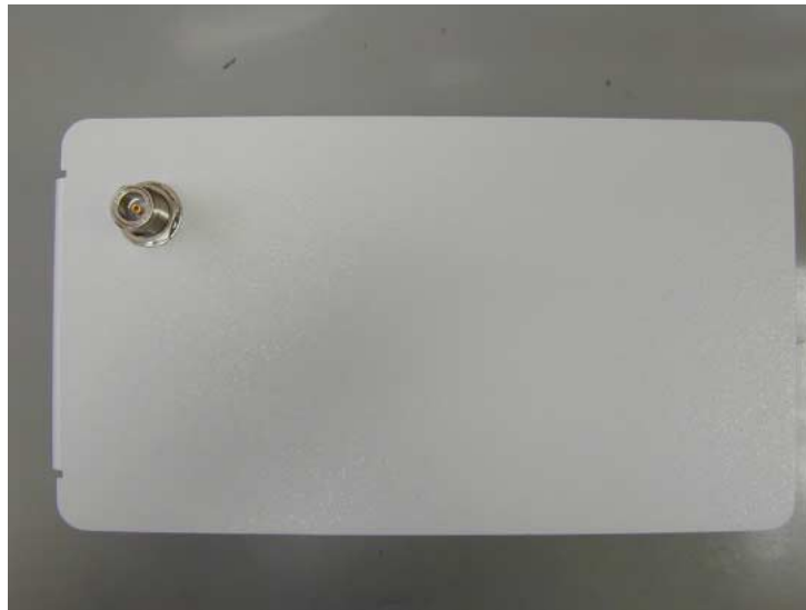
Photo 1. Outdoor unit. External view. Top External antenna
