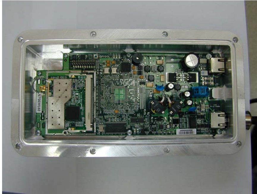
Outdoor unit. Internal view. Component side
