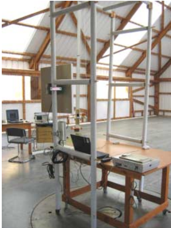
Photograph No.7 Radiated emissions measurement setup at the OATS with double ridged guide antenna
