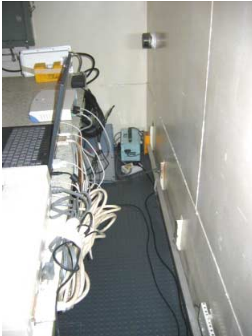
Photograph No.9 Conducted emissions measurement setup
