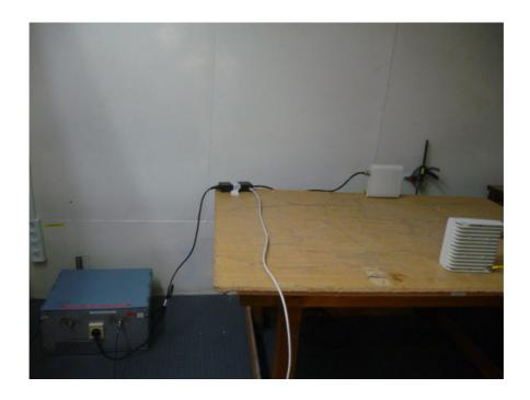
Photograph No.13 Conducted emission measurement setup on AC power lines
