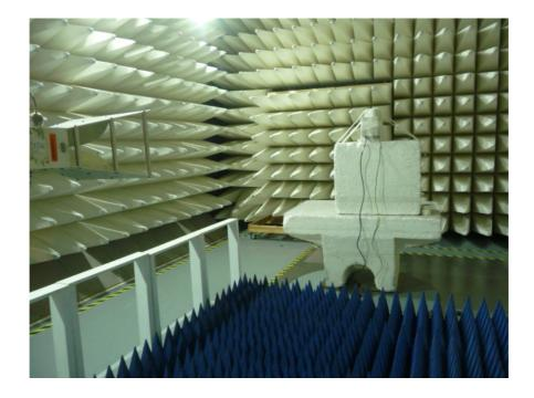
Photograph No.8 Spurious emissions measurement setup in the anechoic chamber in 18-40 GHz
