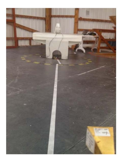
Photograph No.1 Peak output power measurement setup at the OATS
