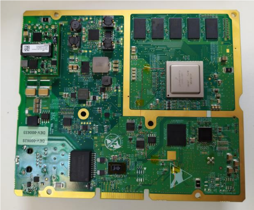
Photo 2 – Digital Control Board (bottom)
