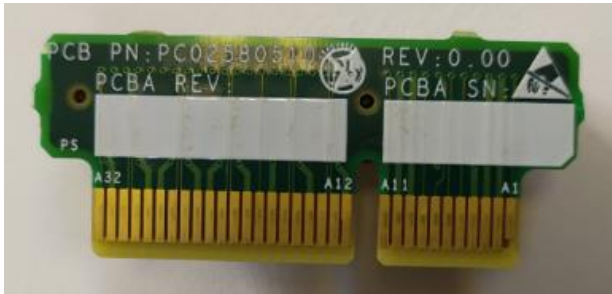
Photo 7 – PCI-e 64 Pin Adapter (bottom)
