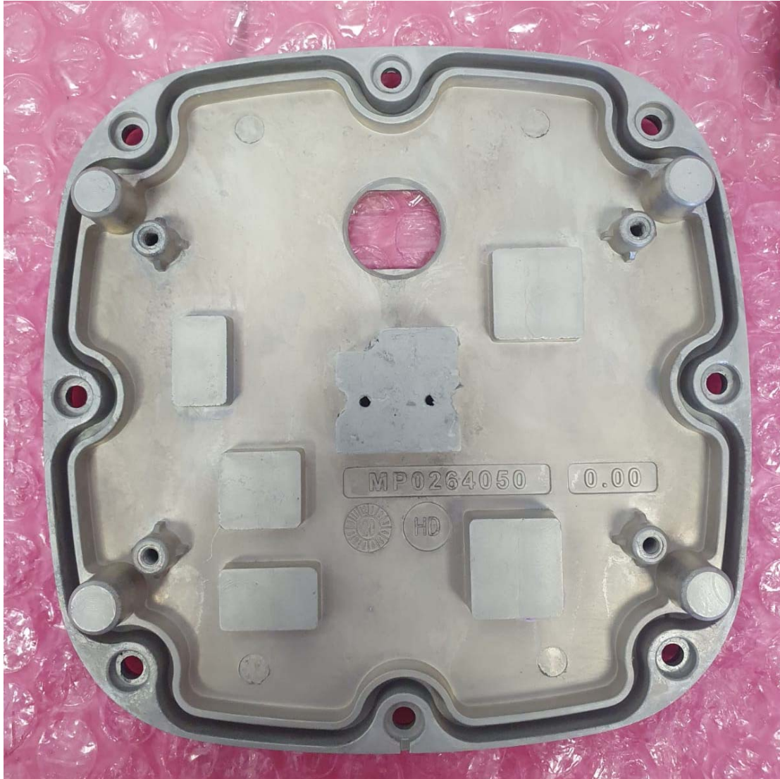
Photograph No.6 RADWIN 6000 6C00 transceiver case internal view
