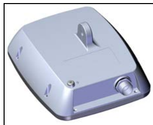
Figure 1-9: SFF subscriber unit with integrated antenna
