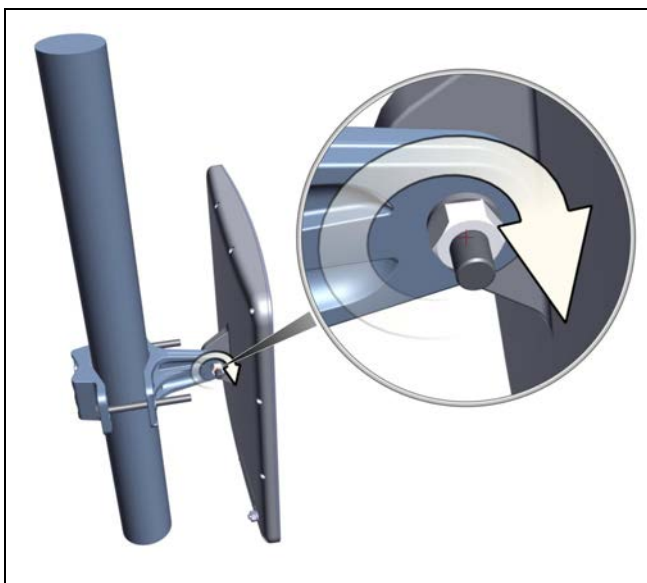
Figure 2-60: Tighten bolt (SU PRO/AIR INT shown)
