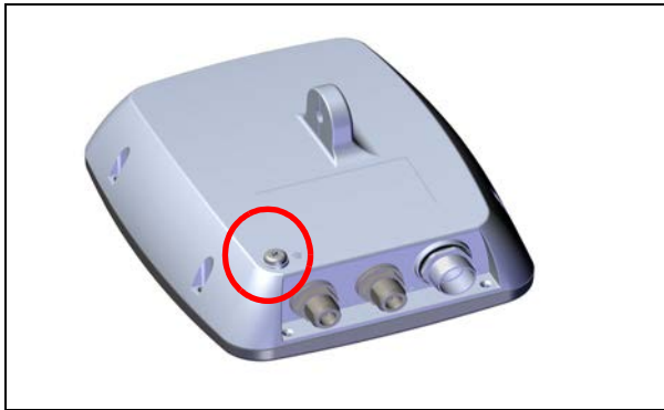
Figure 2-36: Ground: SFF radio unit
