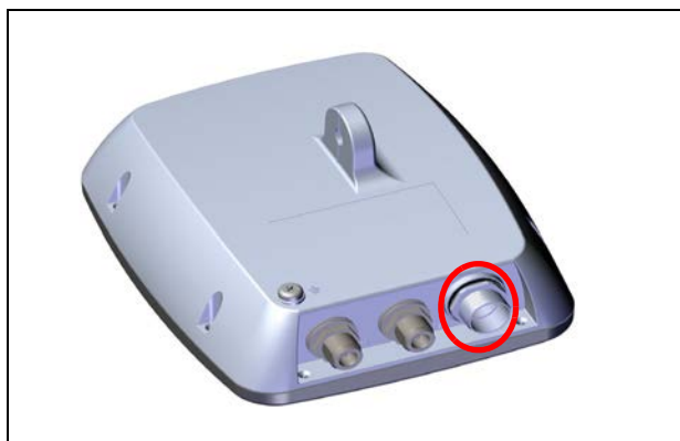
Figure 2-44: Input port: SFF unit (connection label: "IDU")
