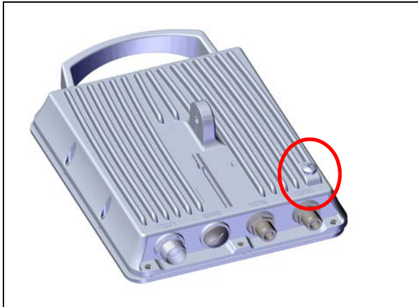
Figure 2-35: Ground: LFF radio unit
