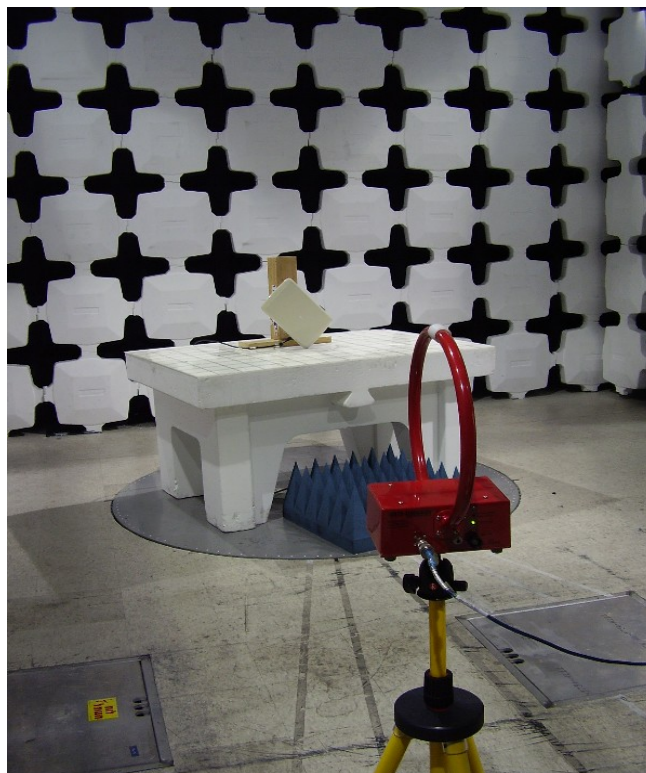
Photo 4. Radiated emission test setup with Loop antenna.
