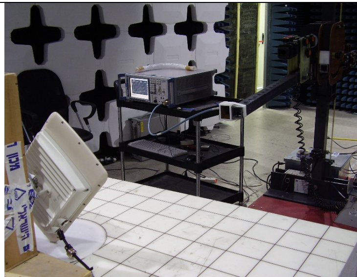
Photo #1. Radiated emission test setup.
