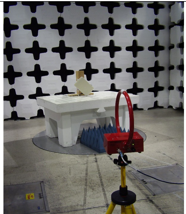
Photo #4. Radiated emission test setup with Loop antenna.
