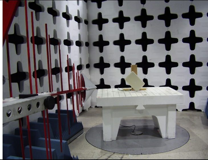
Photo #1. Radiated emission test setup.
