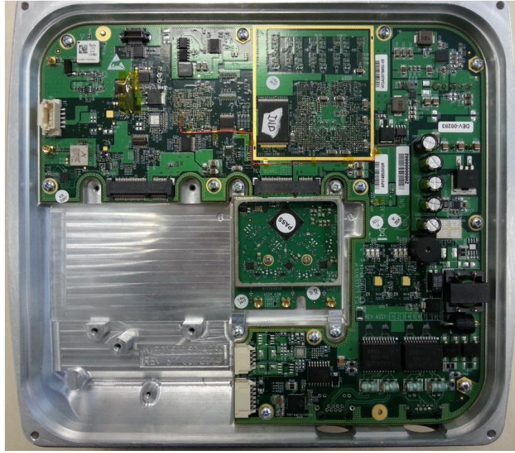
Photo #1: General View of Digital & RF PCBs
