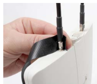
Apply sealing tape - 1
