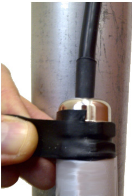
Figure 2-67: Waterproofing an external connection
