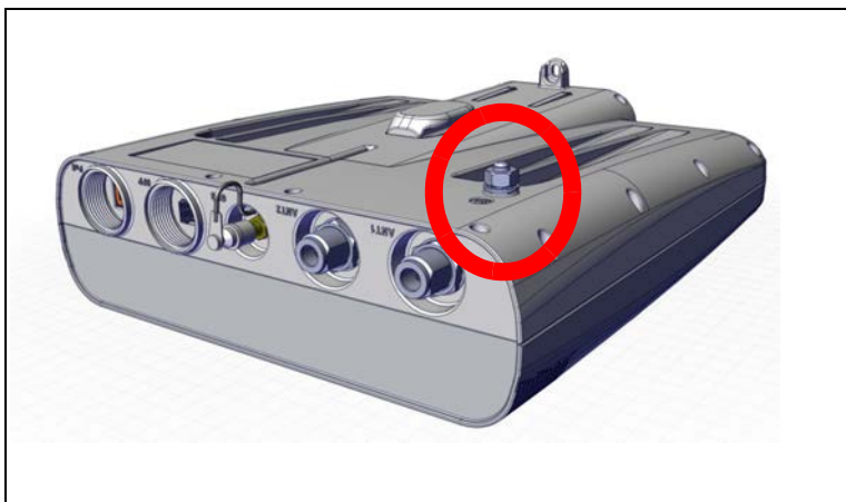
Figure 2-22: Ground: HBS radio unit
