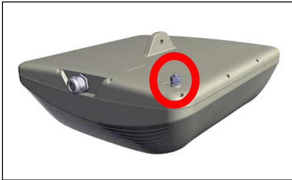
Figure 2-23: Ground: SU radio unit
