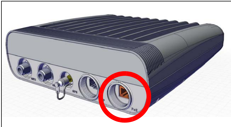
Figure 2-26: Input port: HBS unit (connection label: "PoE")
