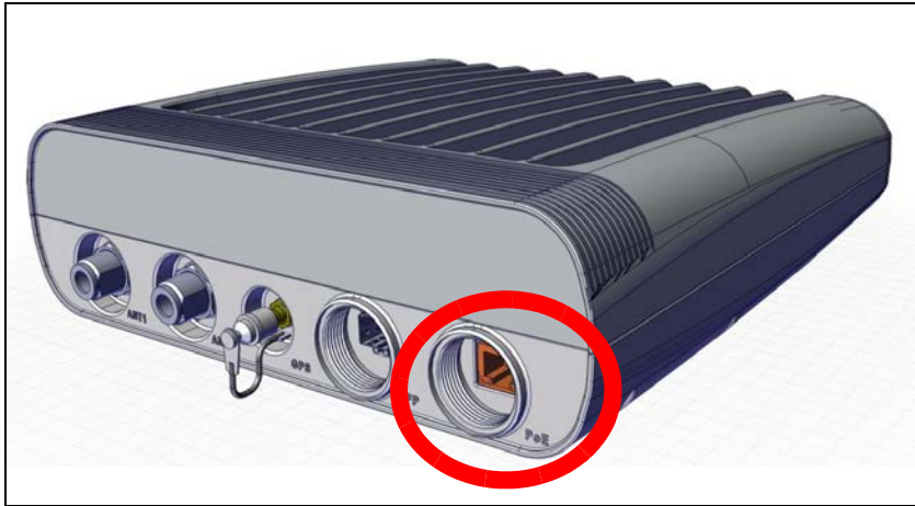
Figure 2-2: PoE port: HBS radio unit
