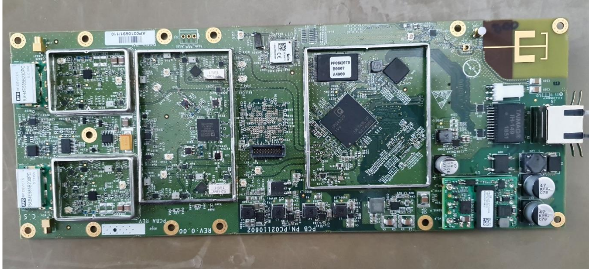
Photo 3: PCB C.S. view with shields off
