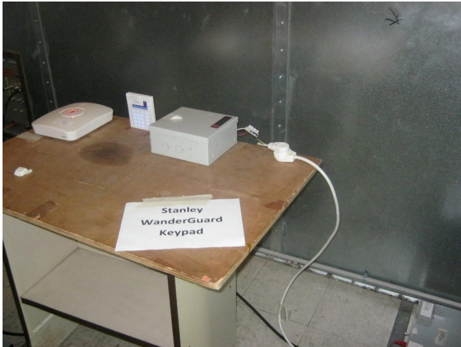
Figure 2. Conducted Emission from AC Mains (AC/DC adapter type 1) Test Setup
