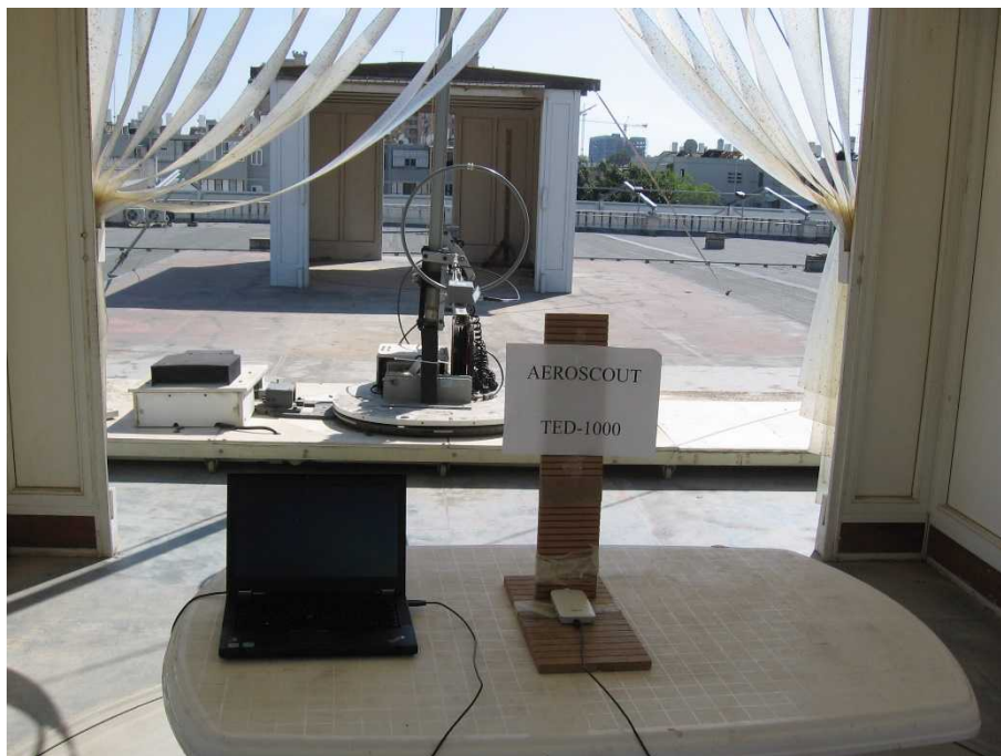
Figure 4. Radiated Emission Test
